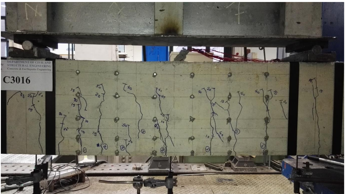
Figure C.13 Final cracking pattern in constant moment zone in beam C3016.
