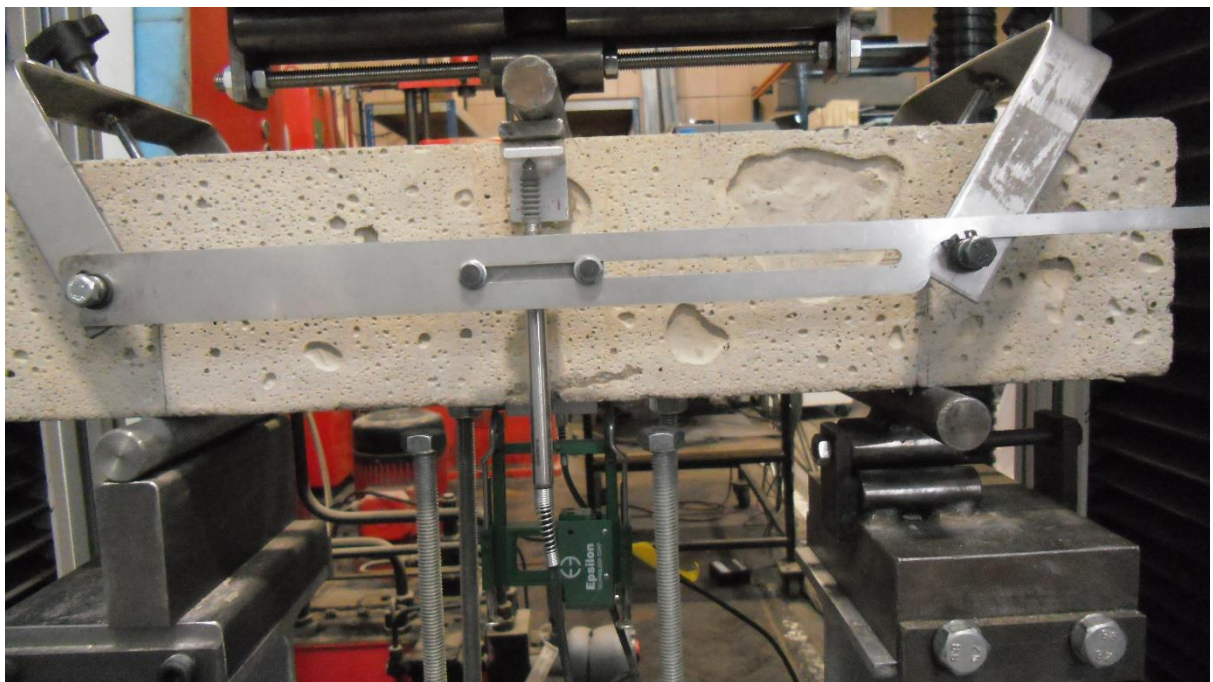
Figure A.10 Testing of SFRC prisms under three-point bending (closer view).
