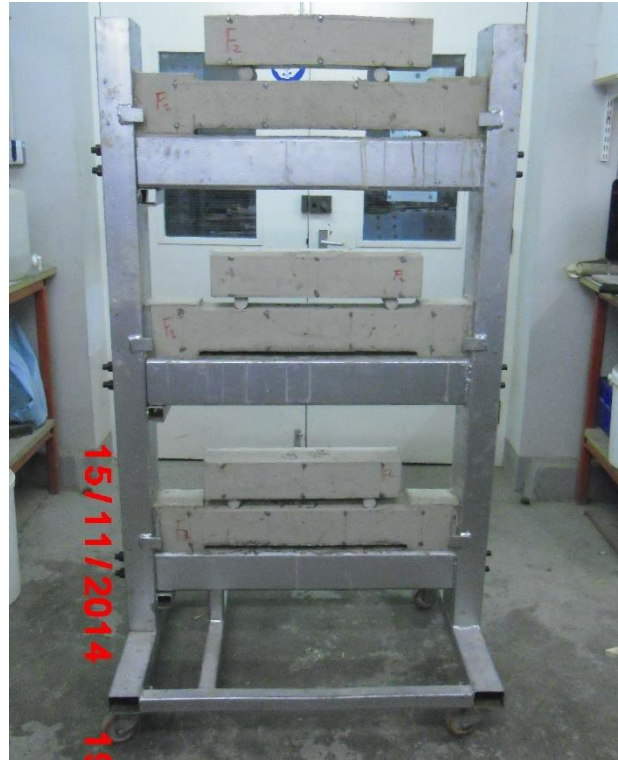
Figure A.3 Free and restrained concrete elements after casting.
