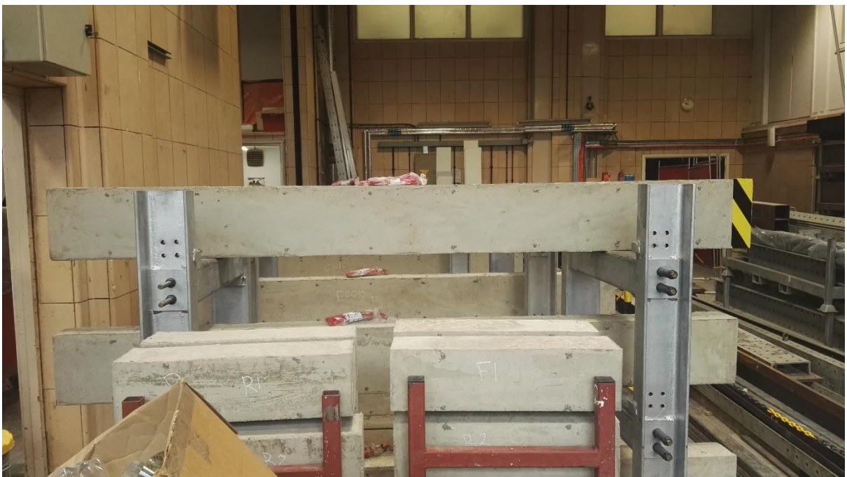
Figure B.4 Distribution of DEMEC discs on beams and prisms.
