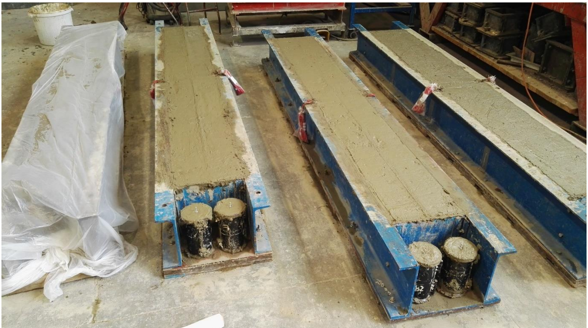
Figure B.2 Moulds after casting.
