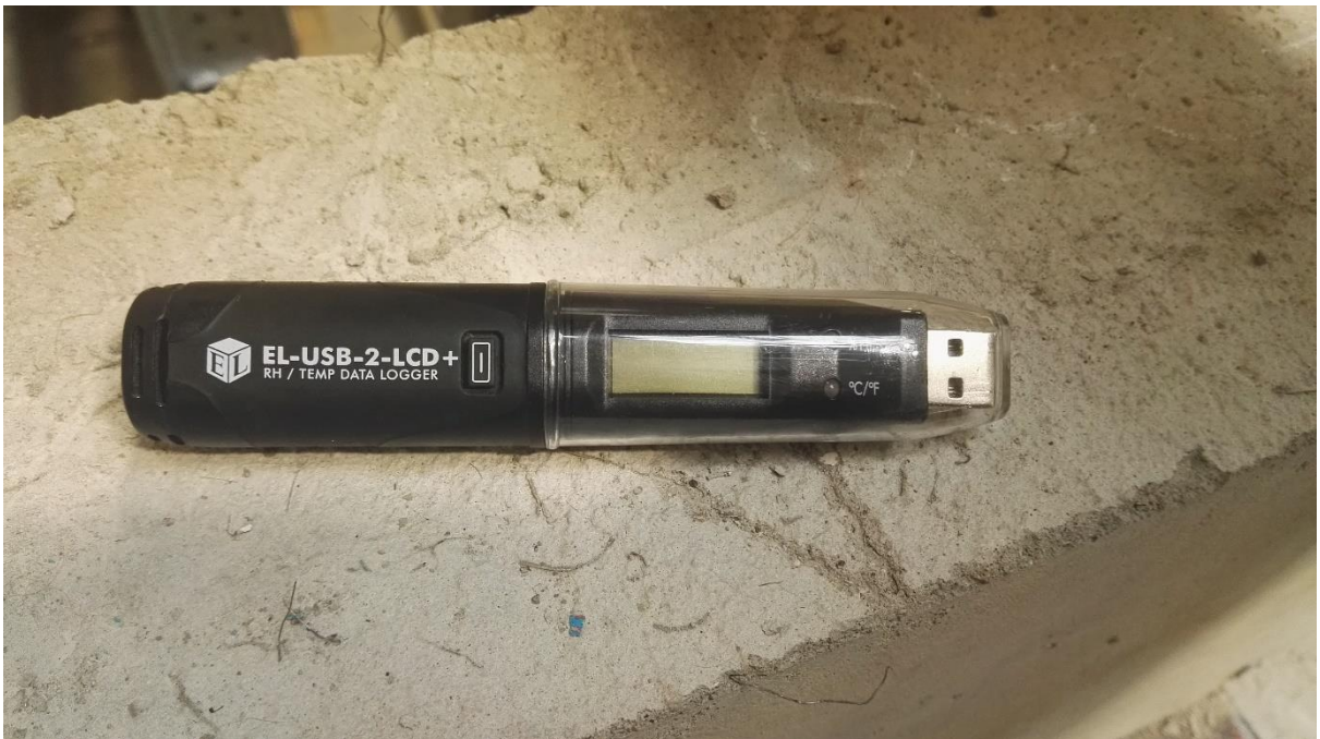
Figure B.6 Used USB device to record ambient temperature and relative humidity during shrinkage measurement period.
