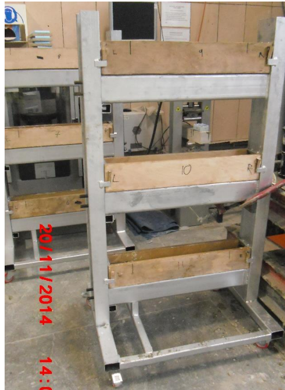
Figure A.1 Restraining frame before casting.
