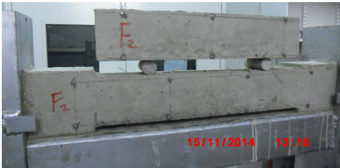
Figure A.4 Detailed locations of DEMEC discs in free and restrained concrete elements.
