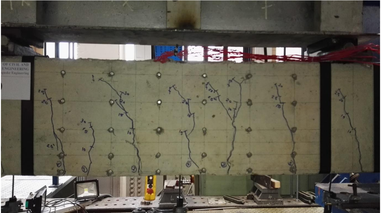
Figure C.12 Final cracking pattern in constant moment zone in beam C3010.
