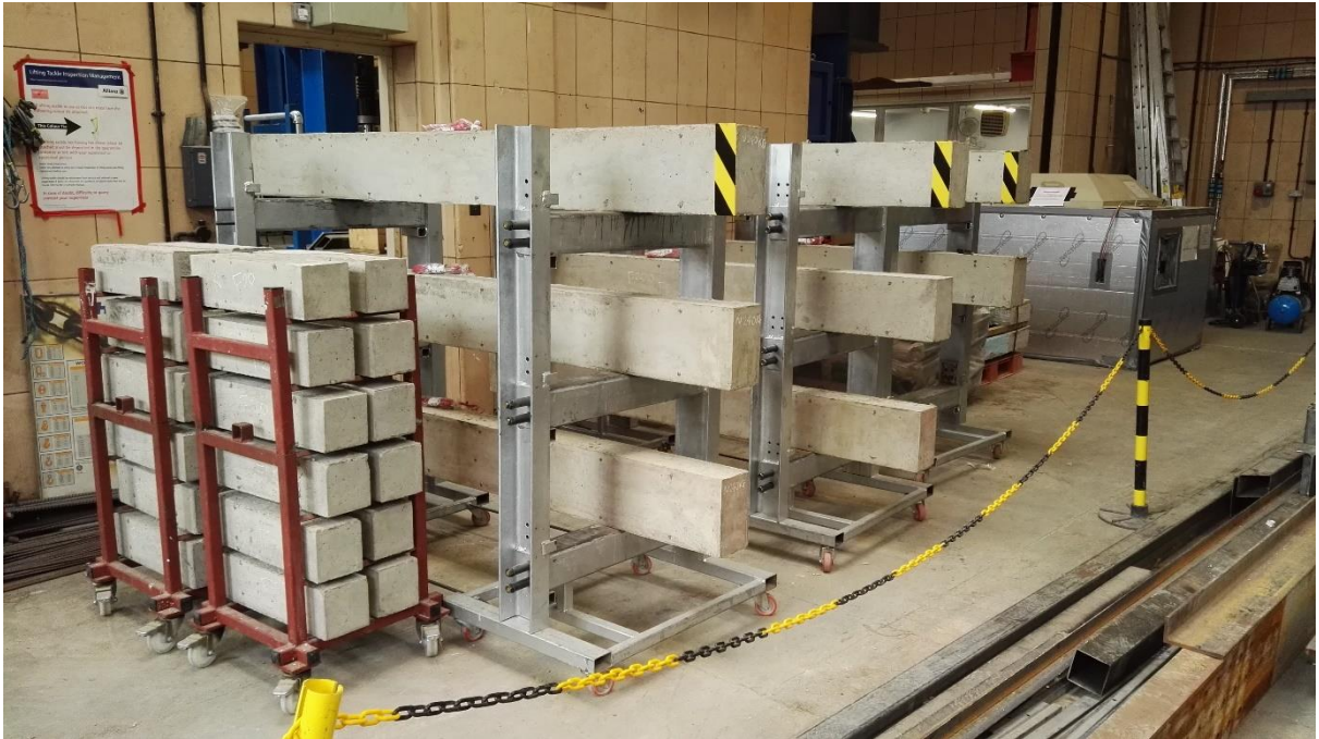
Figure B.3 Plain and reinforced concrete specimens after demoulding.
