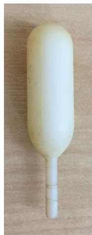
Figure 5.11 The mould for the fabrication of an external latex membrane.
