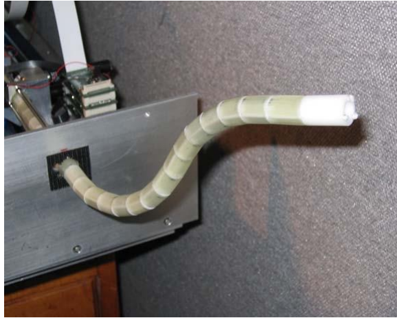
Figure 2.5 Highly articulated robotic probe prototype [7].
