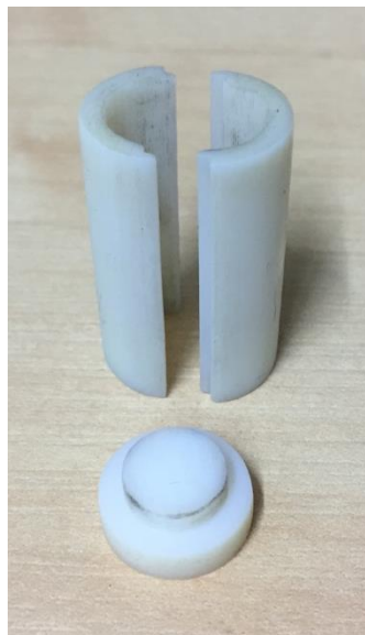
Figure 5.9 Components of the mould for fabricating LMPA-based controllable stiffness element.
