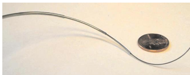
Figure 2.20 Concentric tube robot comprised of four telescoping sections that can be rotated and translated with respect to each other [42]
