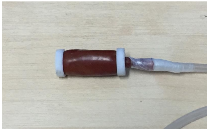
Figure 3.19 Specimen for compression test. The test sample consists a latex membrane and coarsely ground coffee.
