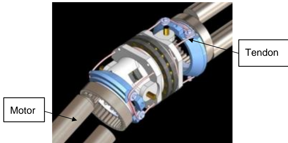
Figure 2.3 3D model of i-Snake articulated joint [21].
