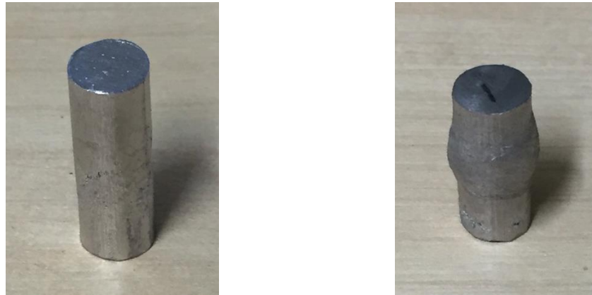
Figure 3.16 Cylindrical specimen before (LEFT) and after (RIGHT) compression test.
