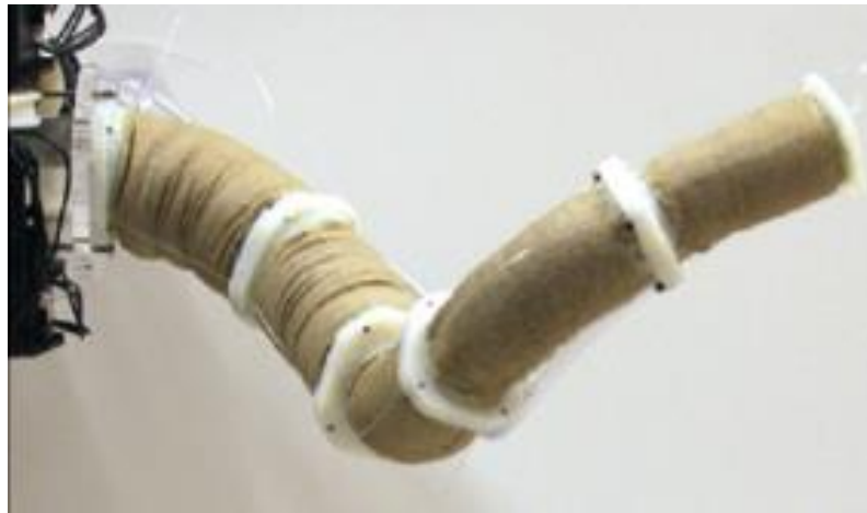
Figure 2.42 Highly articulated manipulator based on granular materials [14].
