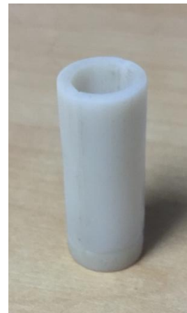
Figure 3.15 Dimension and the prototype of the mould for casting cylindrical specimen.
