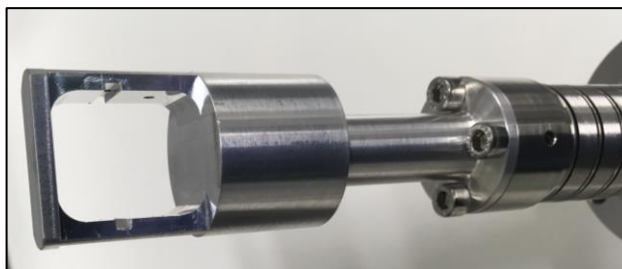
Figure 4.2.13. Image showing the load-lock cartridge holder. Mounted on the 150 mm linear drive.
