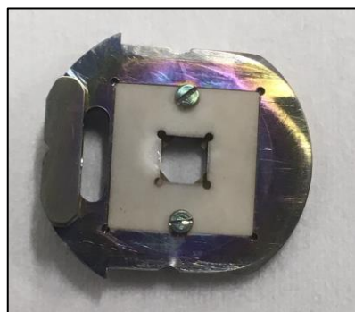
Figure 4.2.11. Image showing the top view of the PLD sample cartridge. The image was taken after several hours of deposition with substrate heating.
