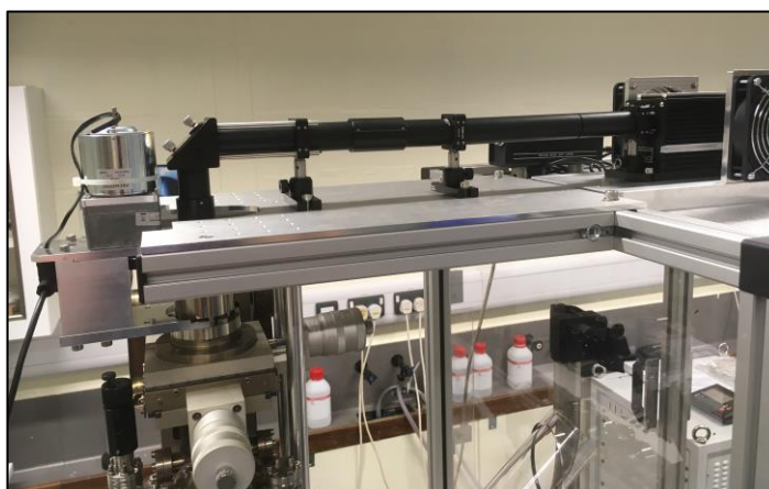
Figure 4.2.21. Image showing the PLD CO 2 laser substrate heating set up.
