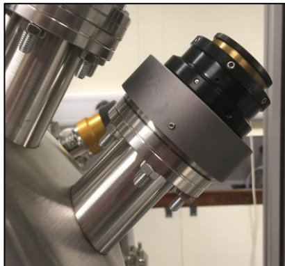
Figure 4.2.6. Image of the Fused Silica lens holder, mounted onto the fused silica viewport.
