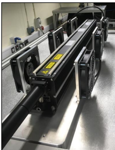
Figure 4.2.20. Image of the 48-2 series SYNRAD CO 2 laser, mounted on the cooling base.
