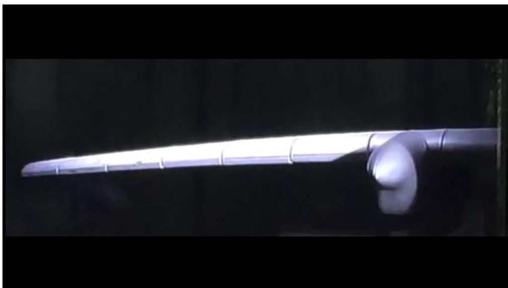
Figure 6.5: Front view: Present wing set-up in a wind tunnel as the right wing [145]
