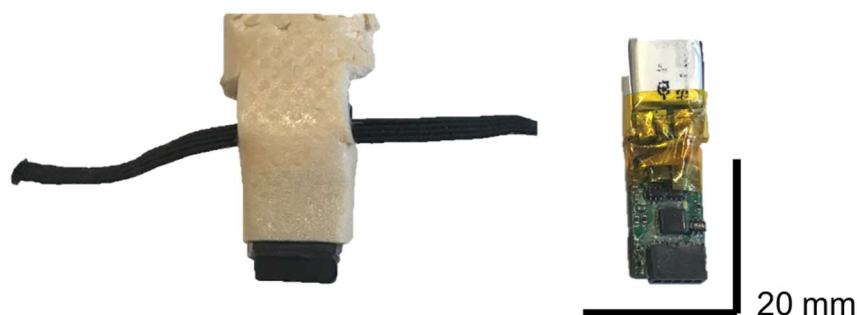
Figure 4.5 Photograph of accelerometer and final harness design.
