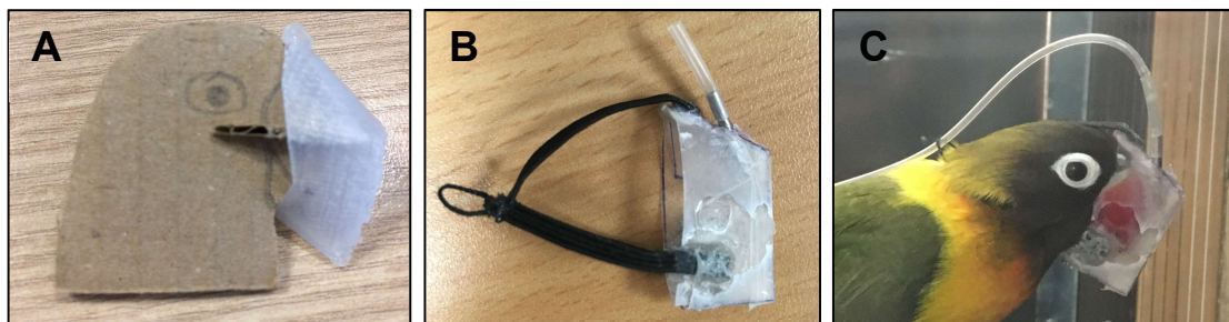
Figure 4.2 Respiriometry masks. (A) 3D printed mask. (B) Cellulose acetate mask. (C) Final cellulose acetate mask with tubing on masked lovebird.
