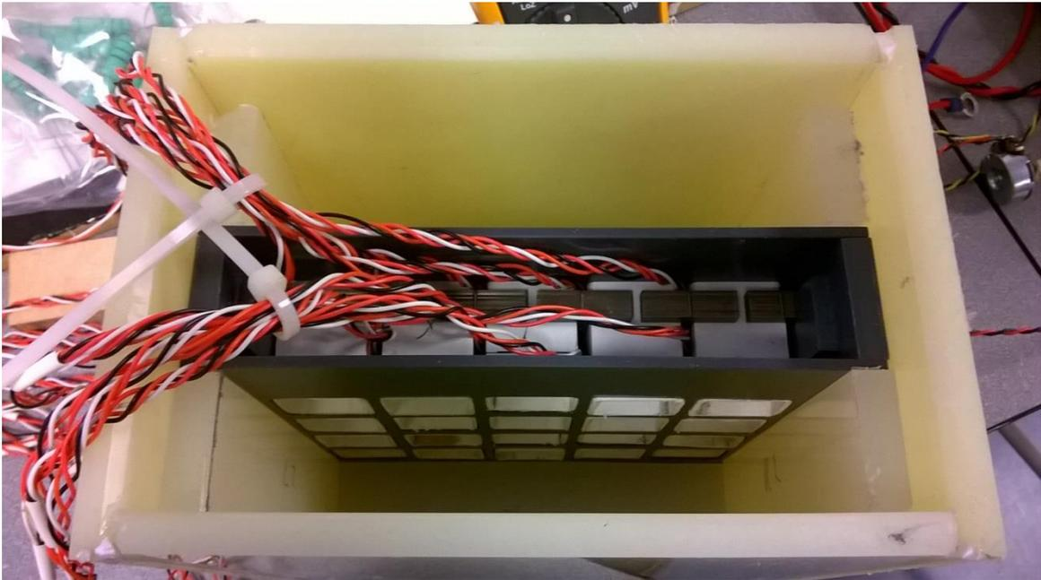
**Figure 3.10 – Flow-through current sensor inserted into test cell case. Electrolyte can freely flow-through the white square tubes which pass through the sensor system.**
