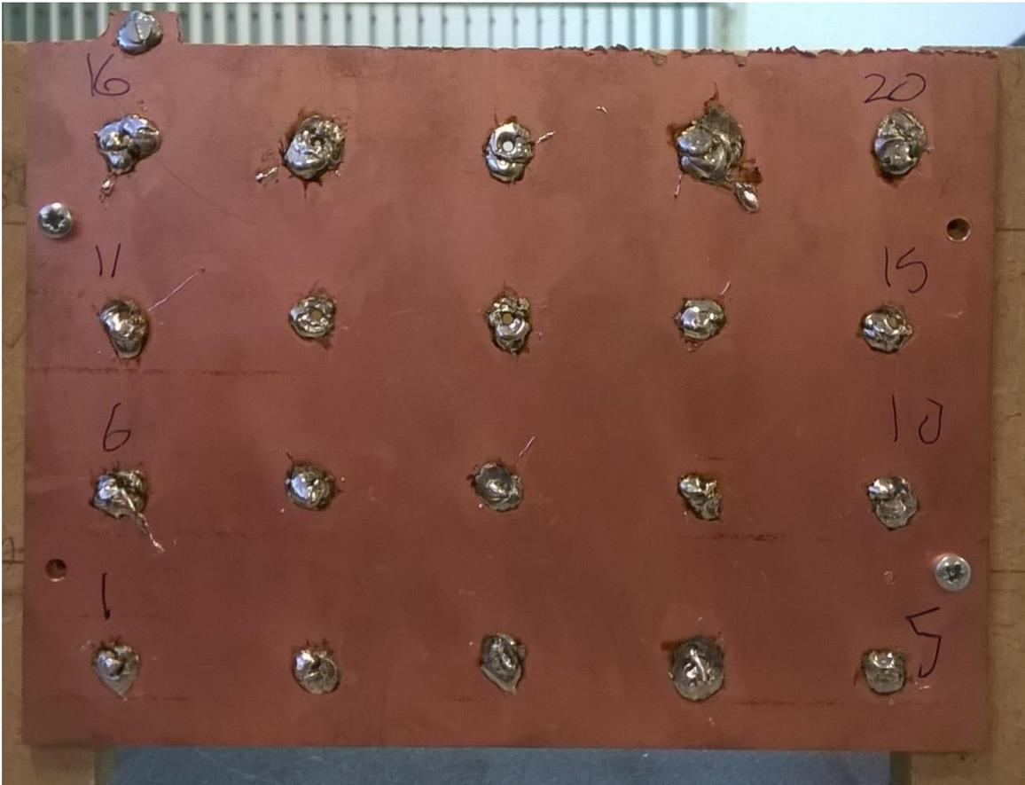
Figure 5.34 – Copper-clad board cut to match Shield 027 plate dimensions. Holes for ‘electrolyte’ wires are numbered 1-20. Plate tab is at top left, terminal may be screwed to the tab.
