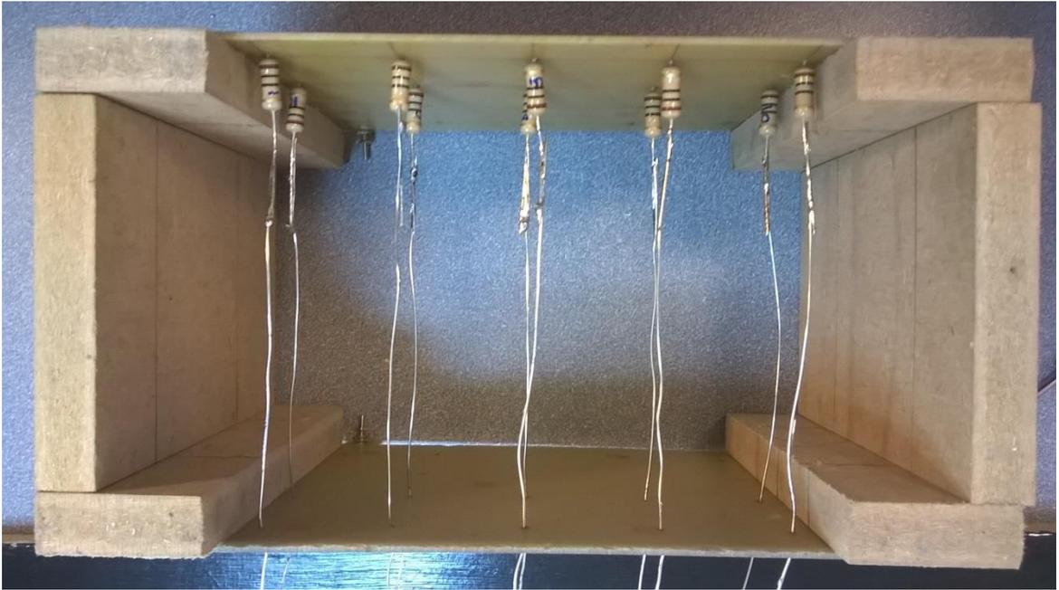
Figure 5.35 –  $10\ \Omega$  resistors used to simulate the electrolyte.
