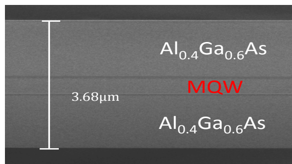
Figure 4.7 SEM image indicating the thickness of the prepared sample
