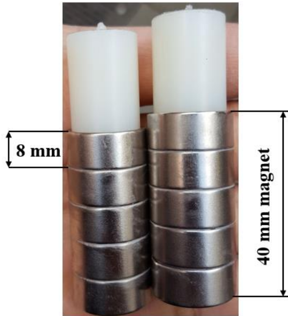
Fig. 5.5: Five 8 mm magnet rings stacked together to form 40 mm magnet.
