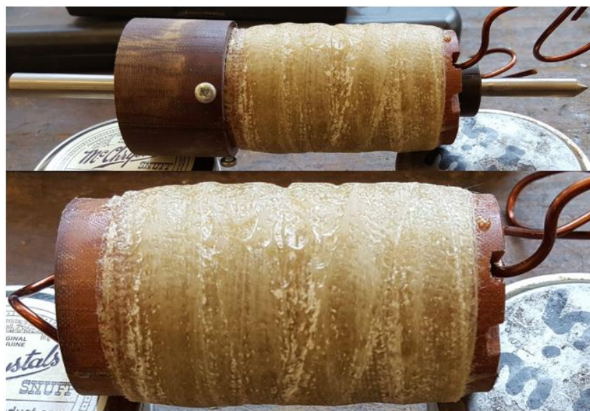
Fig. 5.8: Tufnol outer fixture with fiberglass tape after machining.
