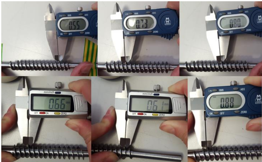
Fig. 5.33: Measuring the width of screw threads.
