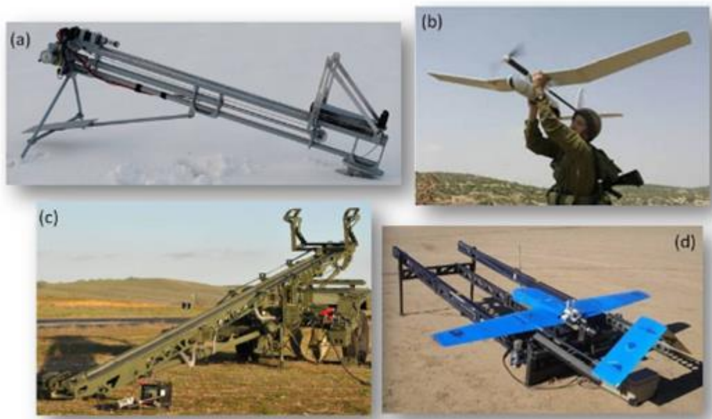
Fig. 6.1: Types of UAV launchers: (a) mini-launcher, (b) hand launching, (c) heavy launcher and (d) universal launcher [20].
