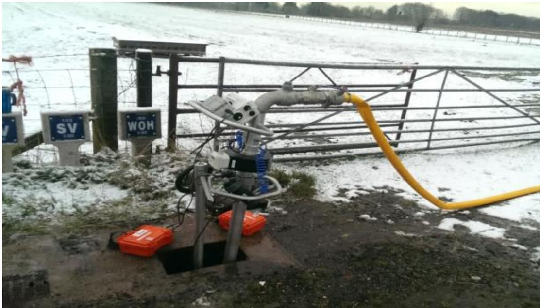
*Figure 39: Monitoring during flow conditioning trials with two ATI NephNet turbidity loggers (orange boxes) and ABB flow meter attached with Langham UK standard standpipe*
