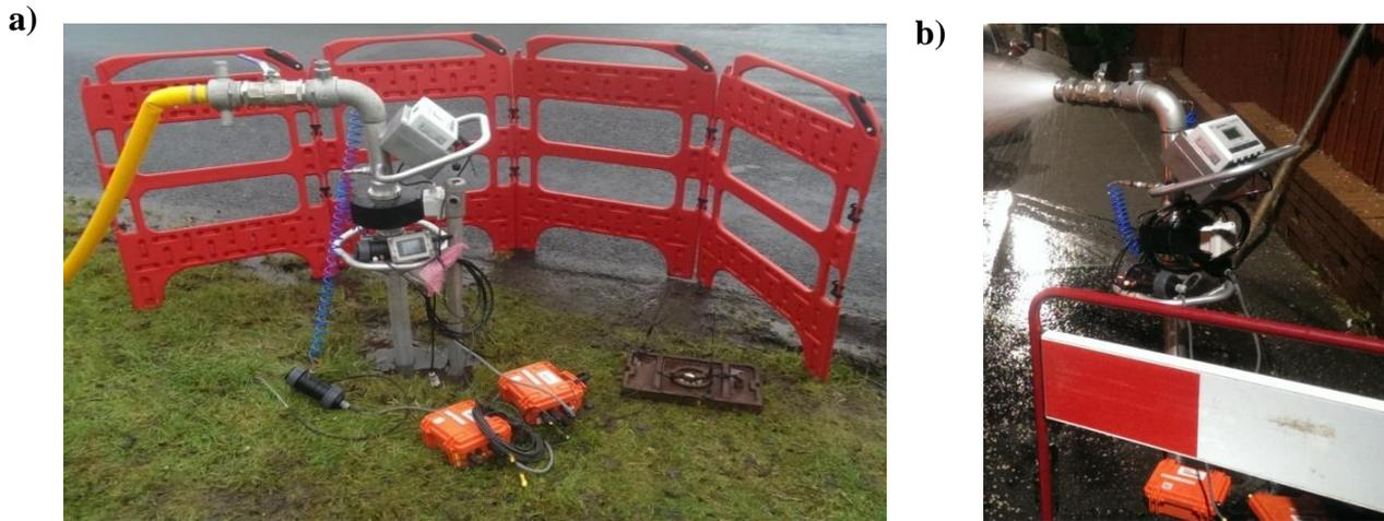
*Figure 9: Intervention operation with the UK specified hydrant standpipe integrated ABB Aquamaster flow meter and turbidity monitoring through twin ATI Nephnet loggers (Turbidity unit included orange boxes and black flow cell) where a) is day time flow conditioning and b) is night time DMA flushing.*
