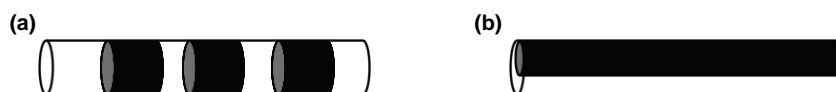
Fig. 1.16 Improper mixing of biphasic reaction in tubular reactors. (a) Segmented flow; (b) density-separated flow
