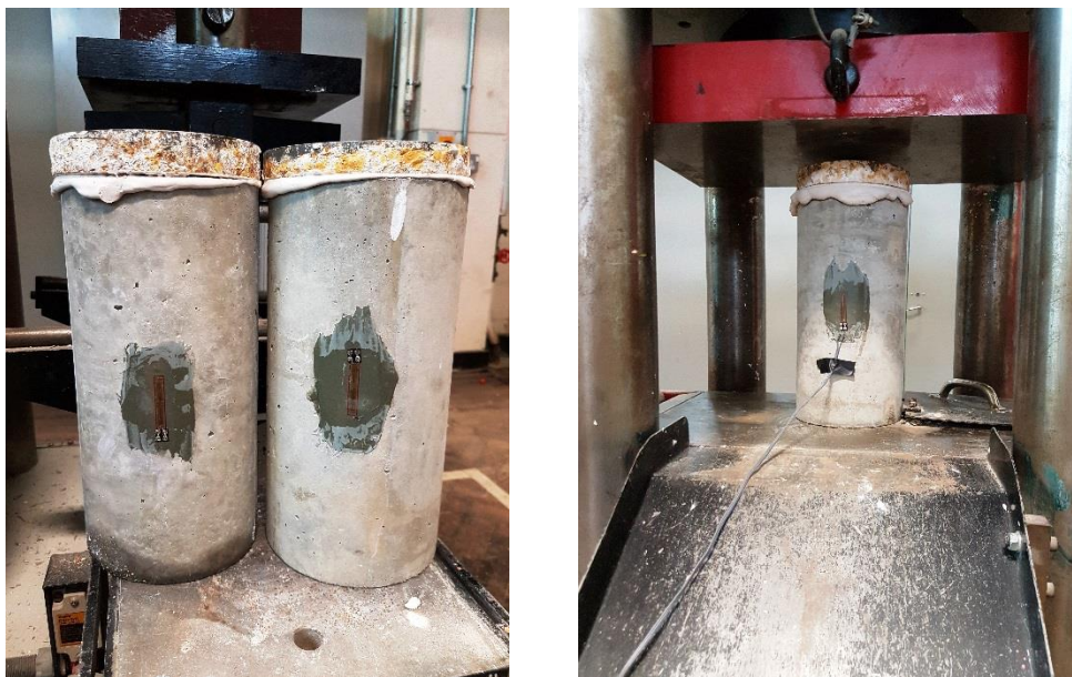
Figure 3.11. Test on concrete cylinders for modulus of elasticity
