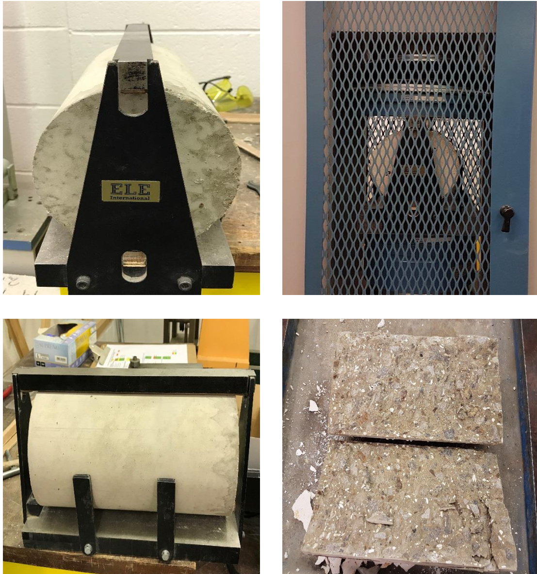
Figure 3.7. Splitting tensile strength test
