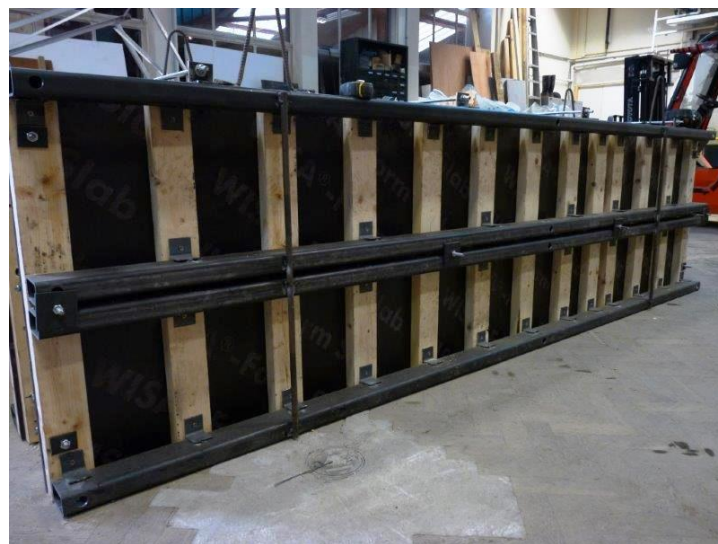
Figure 3.17. Formwork used for casting of the walls
