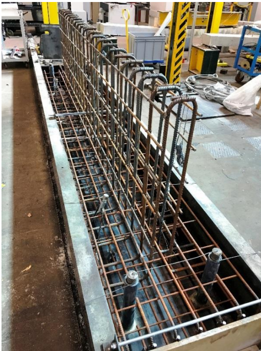
Figure 3.15. Steel reinforcement used in test 4
