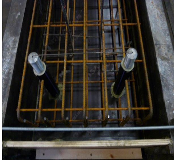
Figure 3.16. Steel studs used for clamping the base slab
