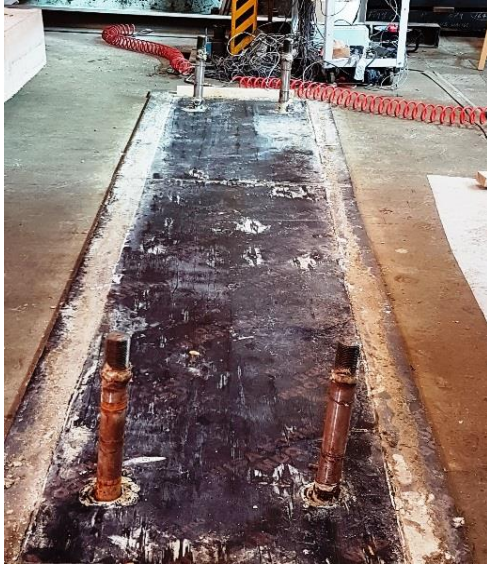
Figure 3.16. Steel studs used for clamping the base slab
