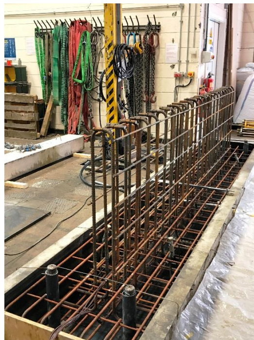
Figure 3.15. Steel reinforcement used in test 4
