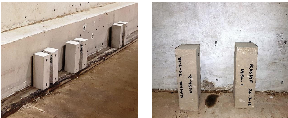
Figure 3.10. Concrete prisms for shrinkage
