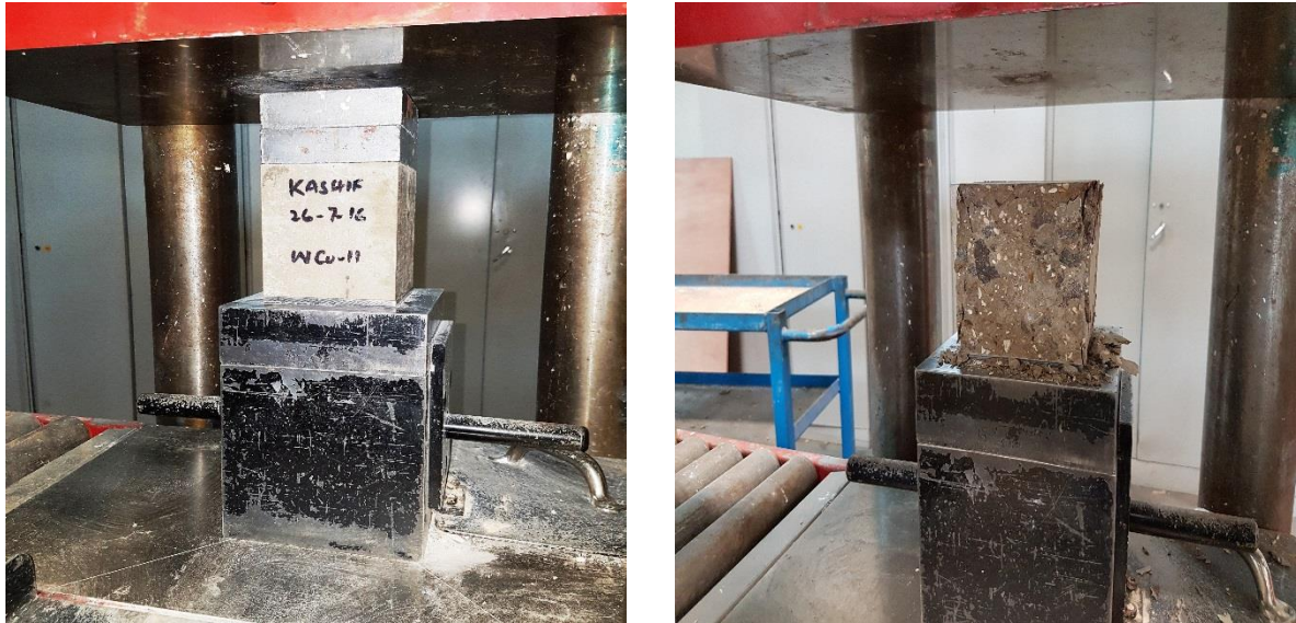
Figure 3.5. Cube tests for compressive strength
