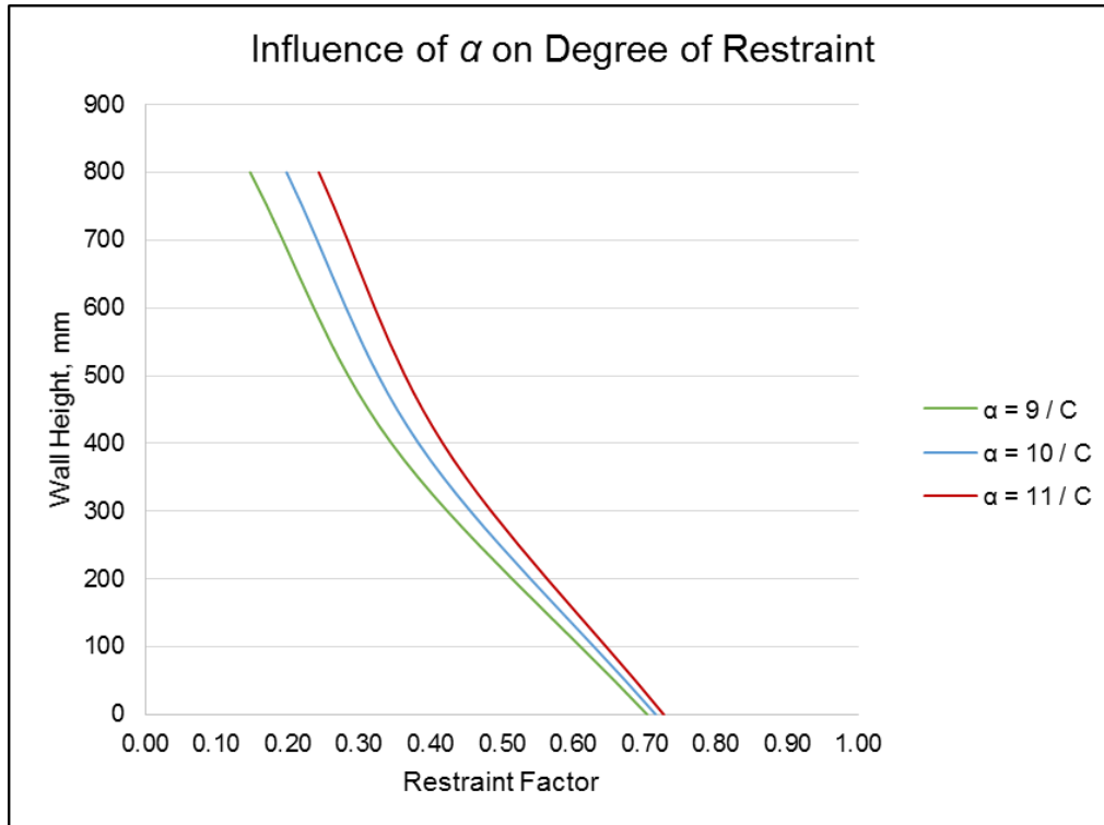
Figure 4.12. Influence of coefficient of thermal expansion on the degree of restraint
