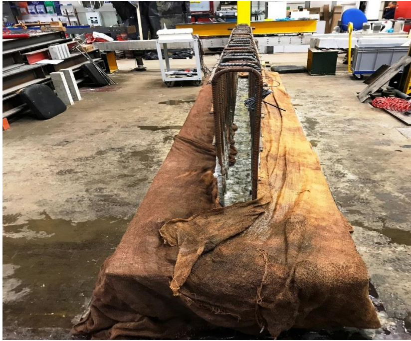
Figure 3.19. Curing of the base slab
