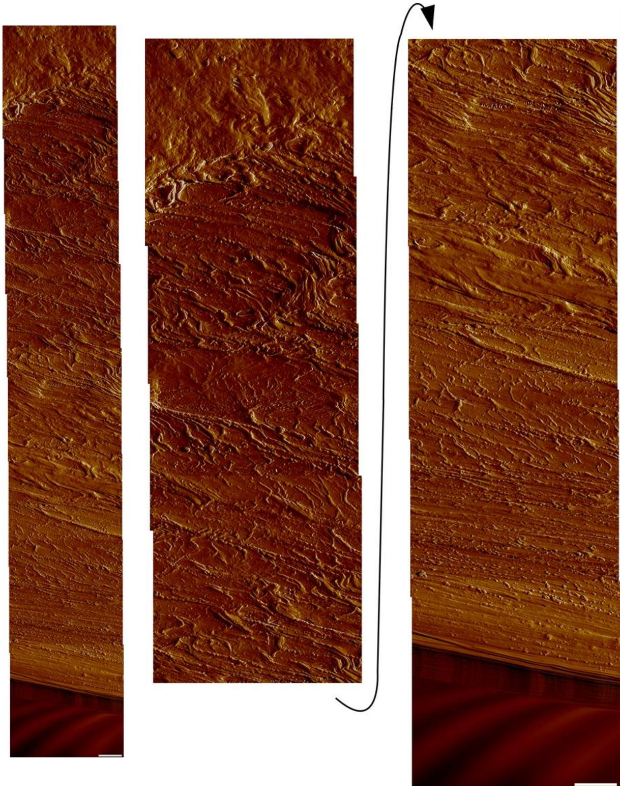
Figure 6.14 – Set of overlapping amplitude images heading towards the crack edge on a crack without a defined white area. Each individual image is 4  $\mu\text{m}$ , scale bar 800 nm. Z scale 500 mv. (Left) set in full, (centre and right) set split in two to see it at a larger scale. Same set as in figure 6.15.
