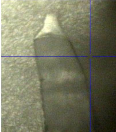
*Figure 6.7 –Optical image of a crack with a white area at the crack tip. The white area is much larger and clearer than in figure 6.1.*
