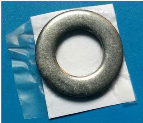
*Figure 7.13 – A frame consisting of a metal washer which is used to keep the film under tension when transferring to another microscope. The white paper seen here was only used in this test.*
