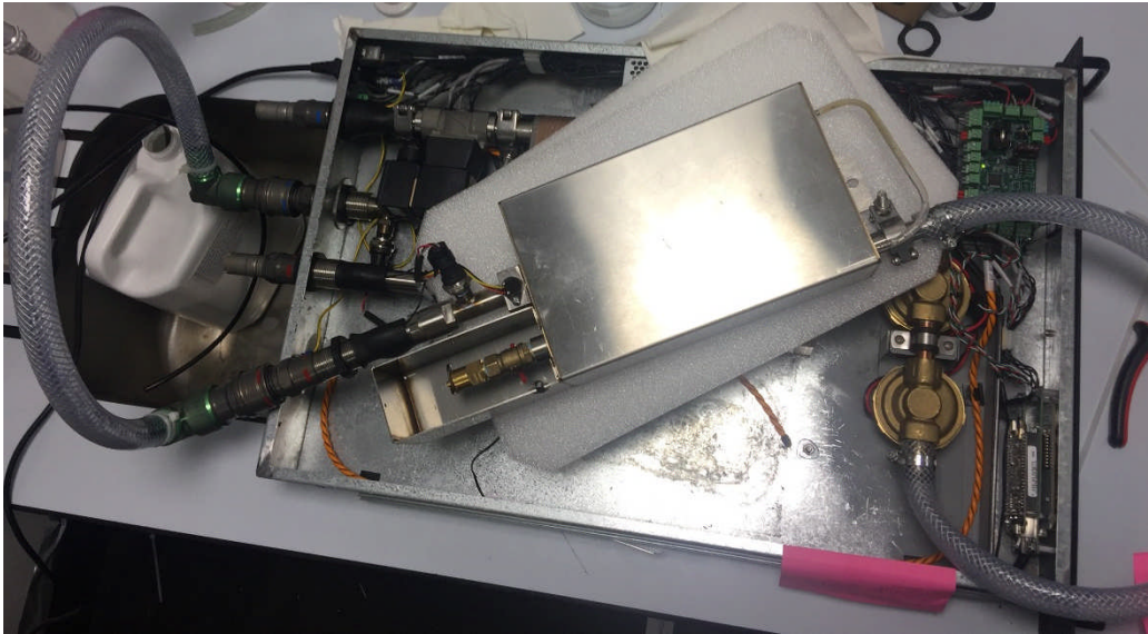
Figure 3.29 A photo showing the CHx40 where the reservoir is placed in a higher level than the pumps and CHx40 is connected via a hose to itself.
