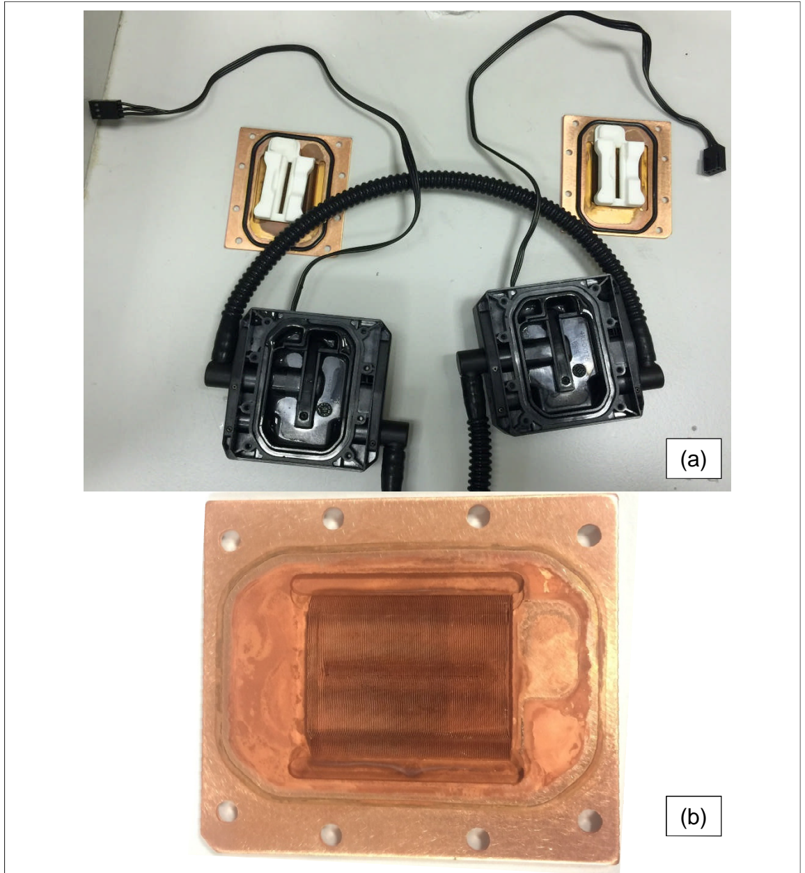
Figure 3.10 (a) DCLC casing from the CPU side showing the cold plate and the attached rubber gasket flow guide and (b) is the V-groove micro-channel cold plate.
