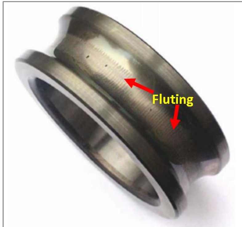
Figure 4.6 Fluting on the inner race (Humbert, 2008)
