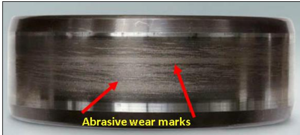
Figure 4.1 Abrasive wear on the bearing inner race (Timken, 2011)
