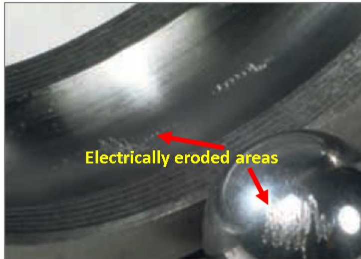
Figure 4.5 Electrical erosion on the outer race and ball bearing (International Organisation for Standardisation, 2017)
