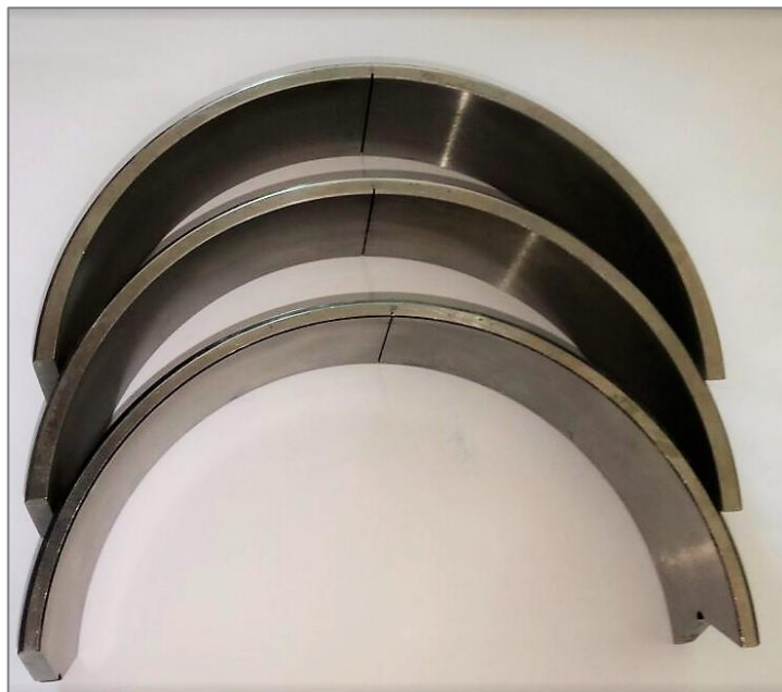
Figure 8.1 Line defects on the bearing outer races
