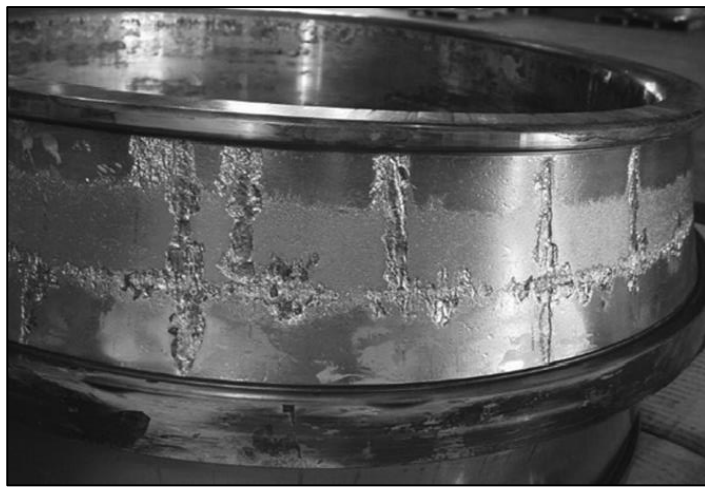
b) Spalling develop into line shape (230/600 series spherical roller bearing inner race) (Kotzalas and Doll , 2010)
