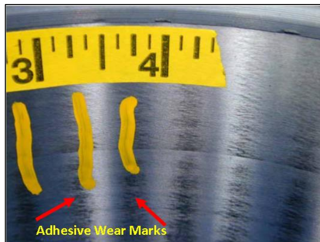
Figure 4.2 Adhesive wear on the inner race (Tallian, 2006)
