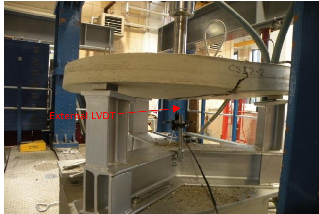
Figure 2-4: Flexural round panel test setup
