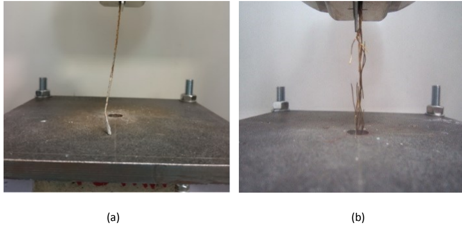
Figure 3-7: Typical failure modes for RTSC: (a) cord pull-out; (b) cord rupture
