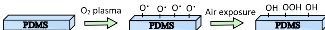
Figure 116. Diagram of the surface of a PDMS substrate during and after plasma treatment.
