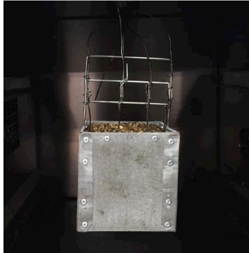
Figure 5.6: Wire mesh basket filled with microwave torrefied sample
