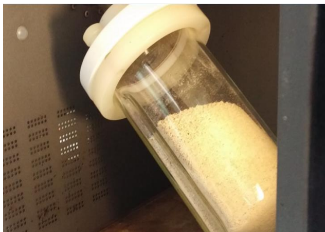
Figure 3.3: Rotating glass flask filled with raw biomass sample inside the microwave chamber
