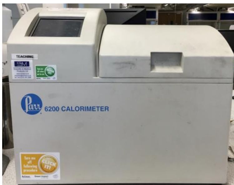
Figure 3.6: 6200 Isoperibol Bomb calorimeter (Parr Instrument Company, USA)
