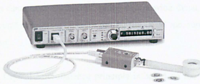
Figure 3.1: Complete QCM set up (QCM200 Digital Controller, QCM25 Crystal Oscillator, Crystal Holder and Quartz Crystal sensors)
