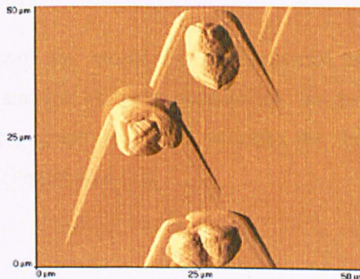
Figure 4.11: Barite morphologies under the treatment of 1 ppm PPCA
