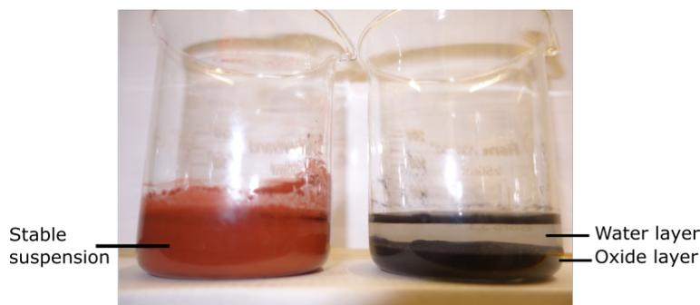
**Figure 6.3:** 50 wt % hematite (left) and magnetite (right), 2 minutes after mixing
