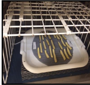
Figure 3-48 Coating Applied Post Freezer Being Inserted Into Blast Freezer
