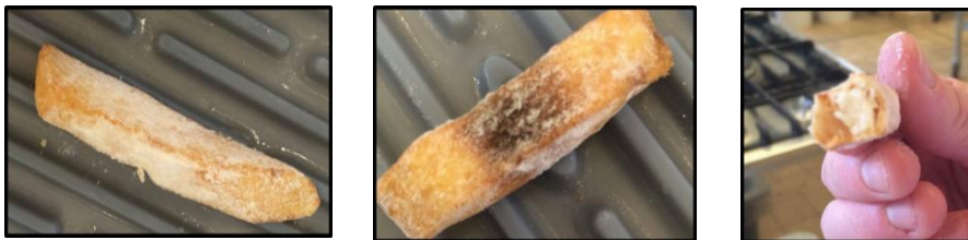
Figure 3-49 Chips Coated with Dry Clear+Stable CRT 30 CMC After Heated in 700W Microwave Oven for 2 minutes 40 Seconds
