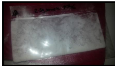
Figure 3-23 3g of Corn Starch Added to Vacuum Bag (90 x90 mm) and Sealed Using Model No. J – V002 Vacuum Sealer from the Food Machinery Company After Application of Paint Roller and Ruler
