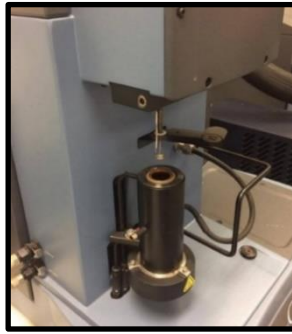
Figure 2-13 Insertion of Sample into Ta Instruments TGA Q50 Model with Inert Nitrogen Flow
