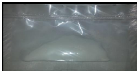
Figure 3-22 3g of Corn Starch Added to Vacuum Bag (90 x90 mm) and Sealed Using Model No. J – V002 Vacuum Sealer from the Food Machinery Company
