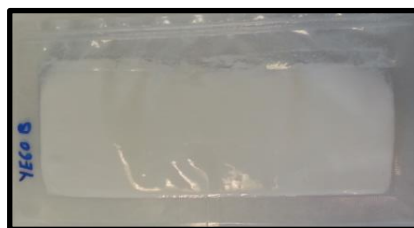
Figure 3-24 2.5g of Corn Starch Added to Vacuum Bag (90 x 90 mm) and Sealed Using Model No. J – V002 Vacuum Sealer from the Food Machinery Company
