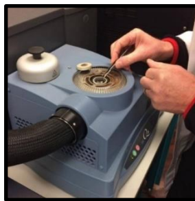
Figure 2-12 Insertion of Sample into DSC Q20 Model with Inert Nitrogen Flow
