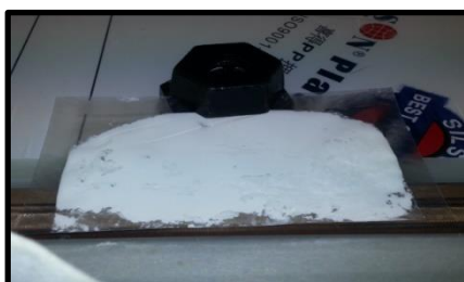
Figure 3-25 Addition of 1kg Weight to 2.5 g Starch Powder Sample Prior to Vacuum Sealing via Model No. J – V002 Vacuum Sealer from the Food Machinery Company
