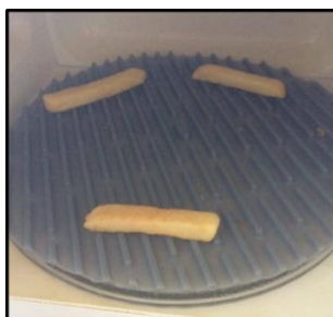
Figure 5-5 Location of the Three Samples Within the Microwave for Every Product and Sample Type
