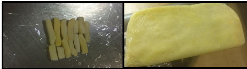
Figure 2-3 Preparation of Uncoated Microchip Inner (Outer Layer Removed) for Insertion into SPDR
