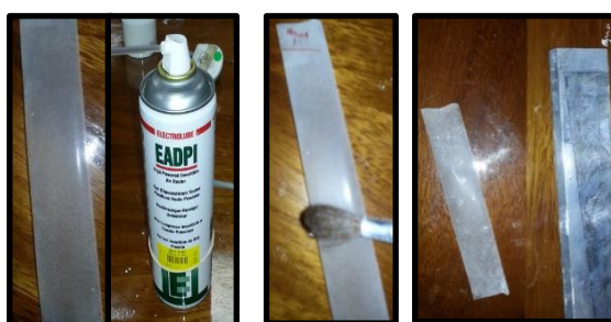
Figure 3-18 Methods Considered as for Adhering Starch Powders to Sellotape Base Material – (l-r): High Pressure Air, Painting Brush, Metal Slider
