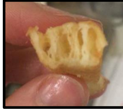
Figure 5-13 Example of a Laminar Structure
