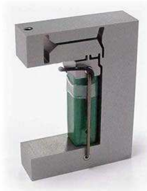
Figure 5.15: The amplified piezoelectric actuator used in the gas valve design. The elastic mechanical amplifier surrounding the crystal stack increases the movement by up to a factor of ten.
