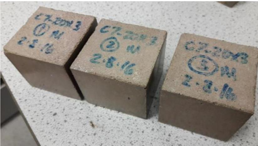
Figure F-8: slag 2 blend under wetting/drying in solution (X3) at 20°C
