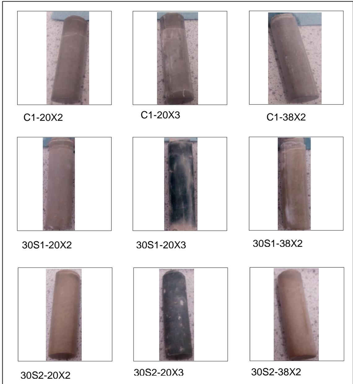
**Figure D-2: Paste samples pre-cured for 28 days before exposure**
