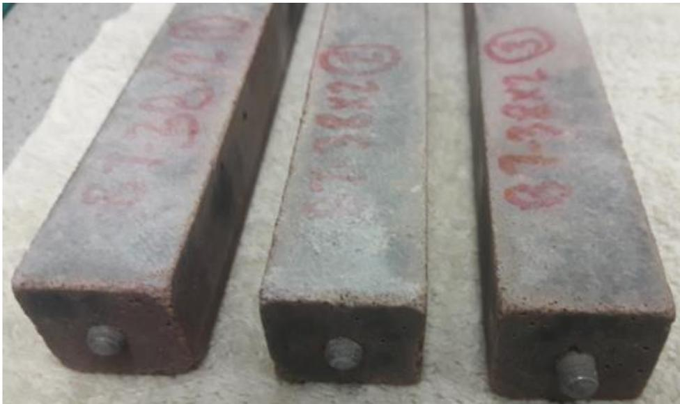
Figure E-6: 30% slag 1 blend submerged in solution (X2) at 38°C
