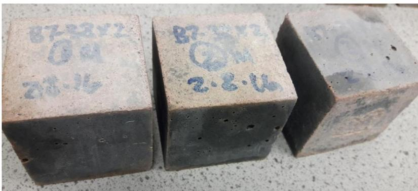
Figure F-6: slag 1 blend submerged in solution (X2) at 38°C
