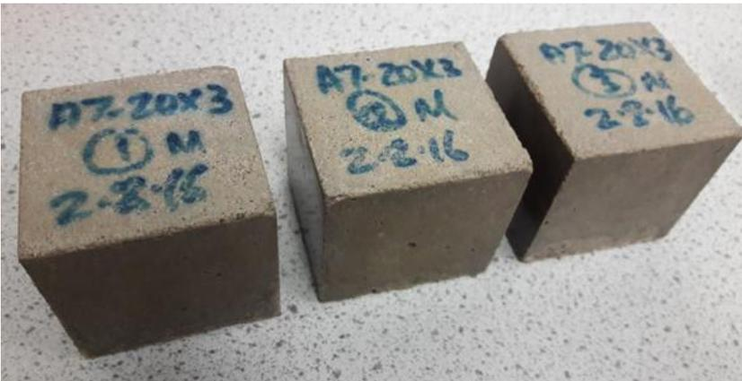
Figure F-2: CEM I cubes under wetting/drying (X3) in solution at 20°C
