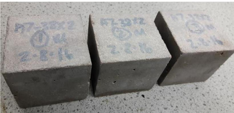
Figure F-3: CEM I cubes submerged (X2) in solution at 38°C
