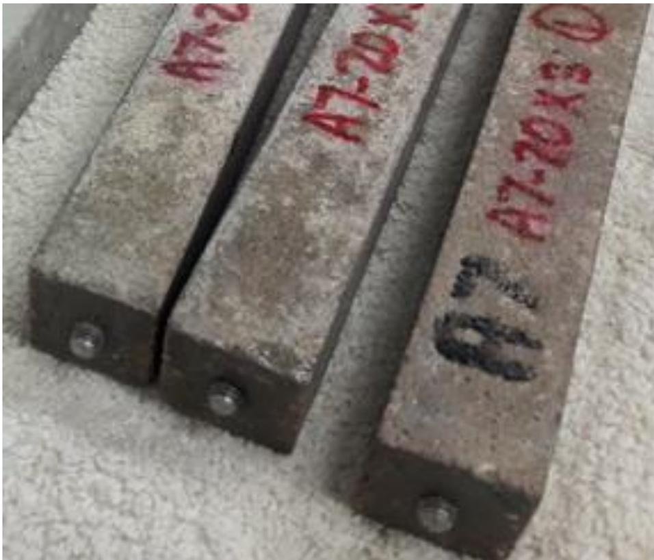
Figure E-2: CEM I prisms exposed to wetting/drying cycles (X3) at 20°C
