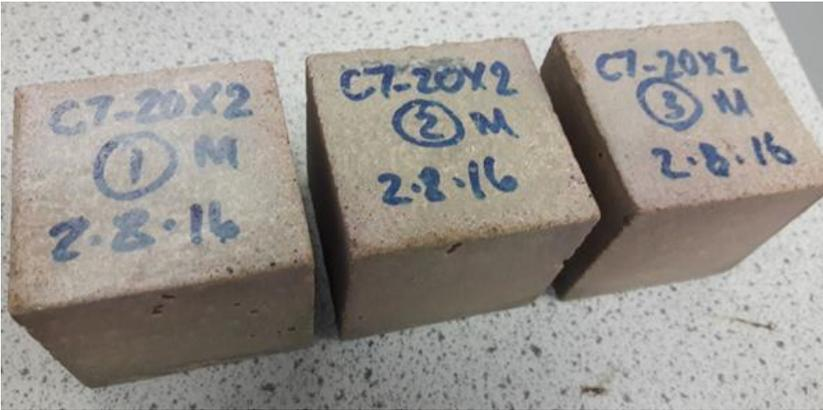
Figure F-7: slag 2 blend submerged in solution (X2) at 20°C
