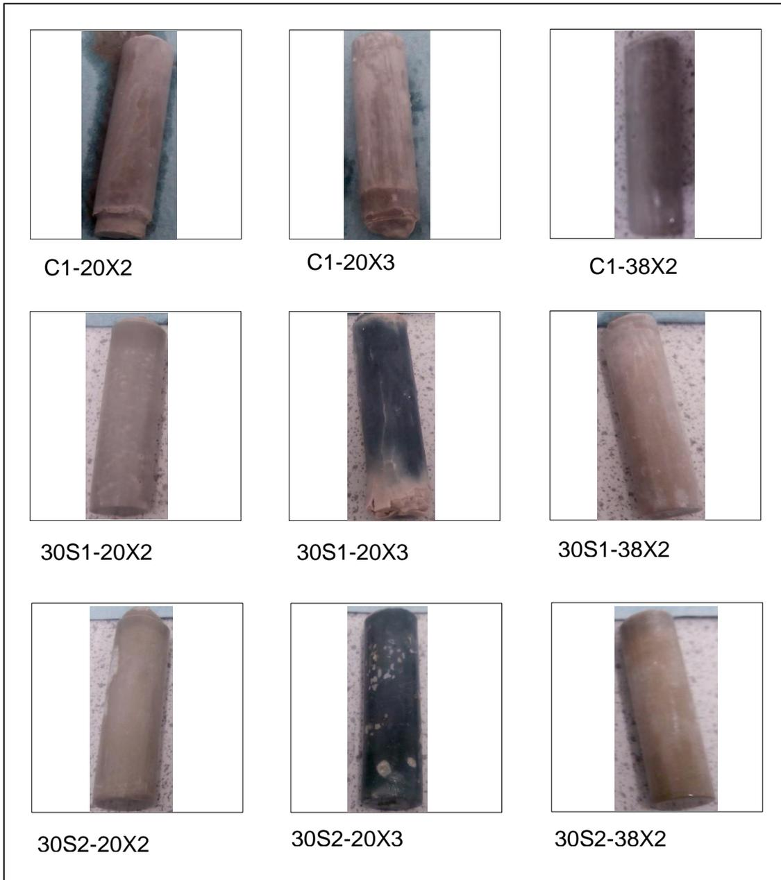
Figure D-1: Paste samples pre-cured for 7 days before exposure
