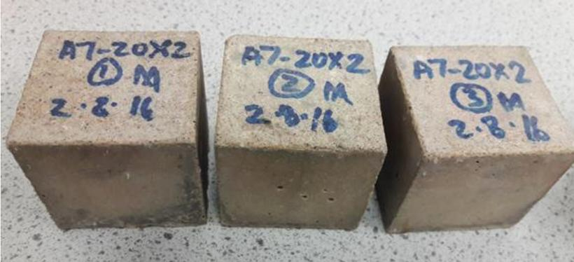
Figure F-1: CEM I cubes submerged (X2) in solution at 20°C
