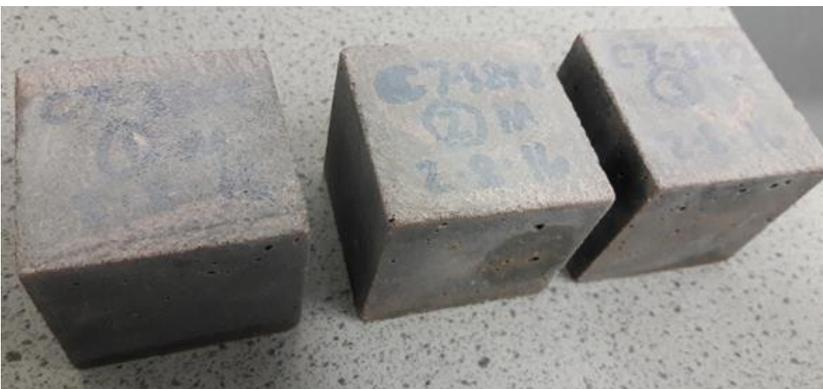
Figure F-9: slag 2 blend submerged in solution (X2) at 38°C
