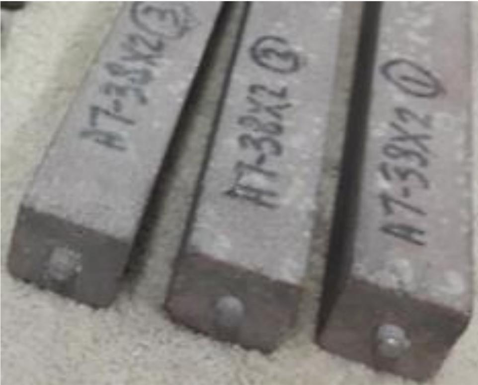
Figure E-3: CEM I prisms submerged (X2) in solution at 38°C
