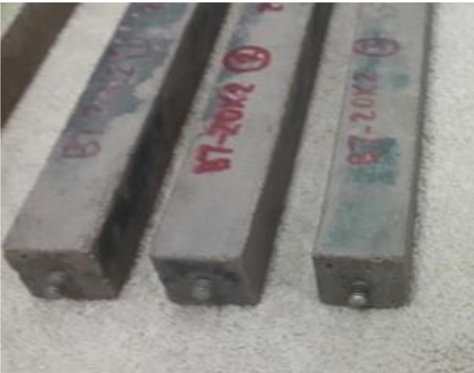
Figure E-4: 30% slag 1 blend submerged in solution (X2) at 20°C
