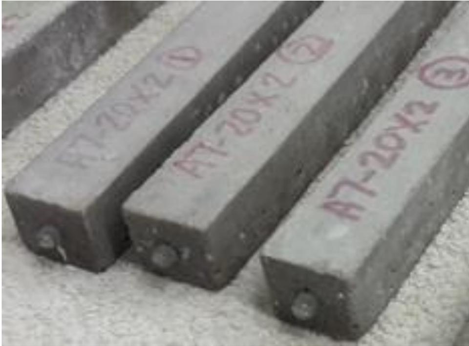
Figure E-1: CEM I prisms submerged (X2) in solution at 20°C
