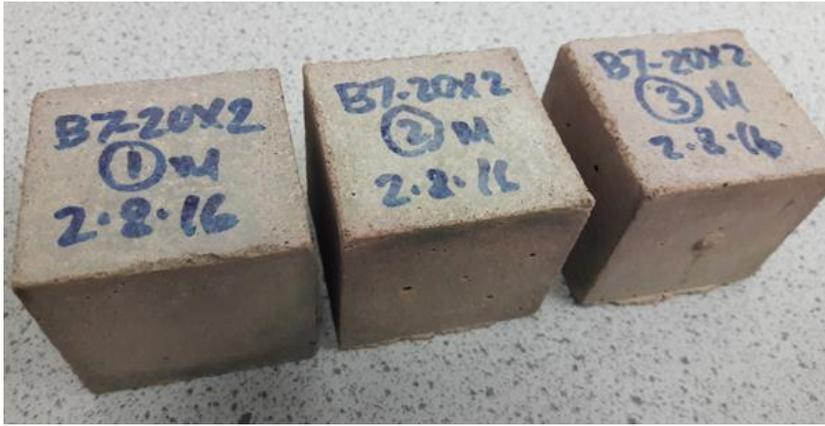
Figure F-4: slag 1 blend submerged in solution (X2) at 20°C
