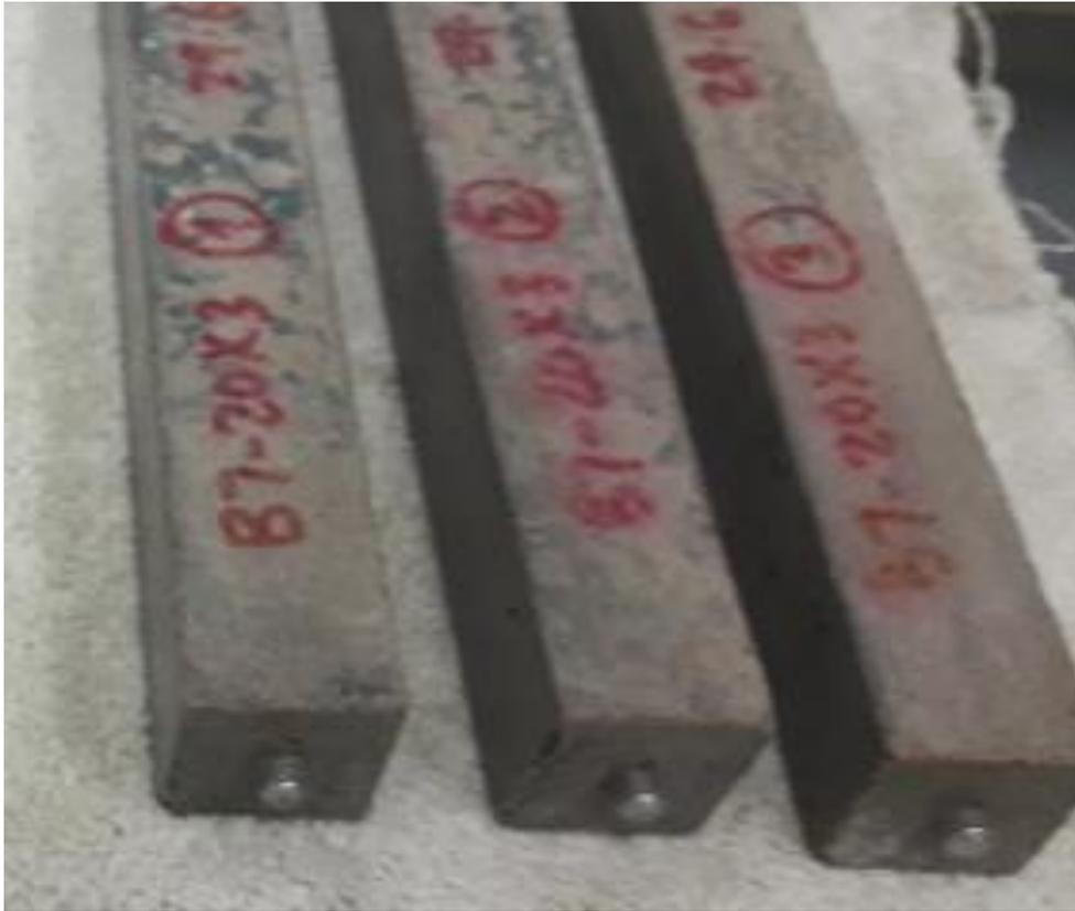
Figure E-5: 30% slag 1 blend under wetting/drying cycles (X3) at 20°C
