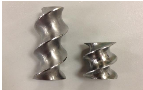
Figure 1-2. Conveying element (left: long pitch conveying element, LPCE; right: short pitch conveying element, SPCE)
