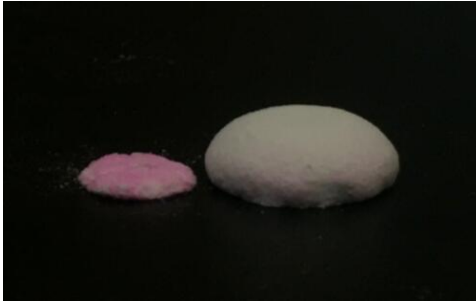
Figure 4-8. Typical nuclei from the compact powder bed (left: MCC; right: lactose).
