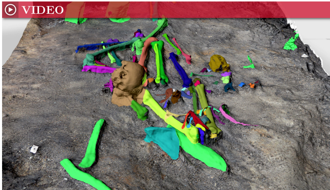
Figure 2.11: (VIDEO) Conceptual illustration of how classification of point clouds and meshes could be done. Also demonstrating preview of online web 3D viewer, which supports selection of classified 3D meshes (in development by the author). Illustration based on data from the Alken Enge excavation (Holst et al. in press).
