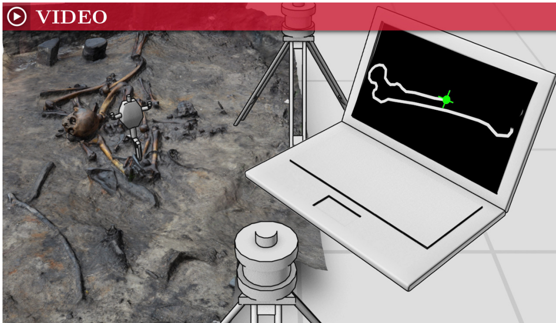
Figure 2.6: (VIDEO) Conceptual illustration of the documentation of an archaeological excavation; real-time 3D vector data acquisition using for example optical ranging with total station or point tracking by radio waves through RF positioning systems. Illustration based on data from the Alken Enge excavation (Holst et al. in press). https://vimeo.com/257346554/1f29c9e930
