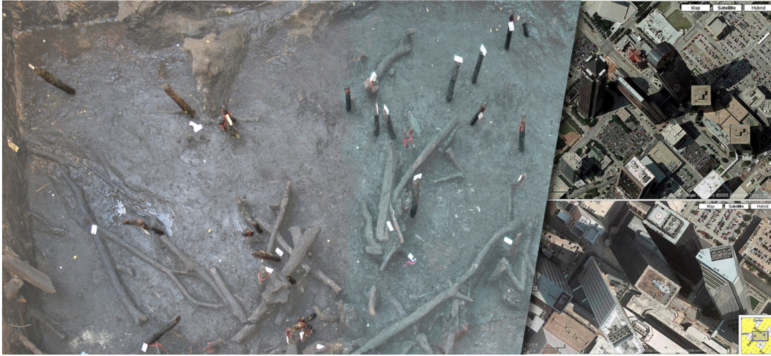
Figure 4.2: A 2D-rectified excavation orthophoto, showing pronounced geometric distortions or "Escher-effects" of protruding wooden structures. The same problem visualised through first-generation Google Earth imagery (Google Maps 2010; Chris Silver Smith).
