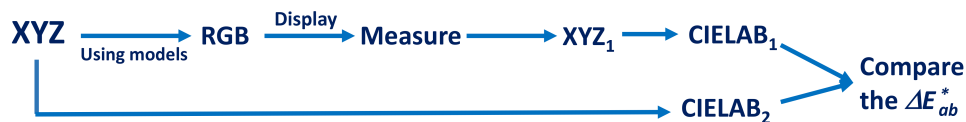
Fig. 3.6 The XYZ conversion procedure and comparison between the target XYZ and measured XYZ .
