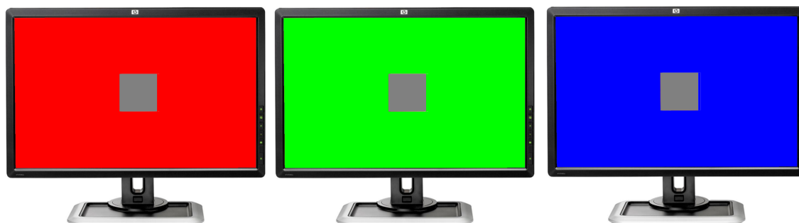
Fig. 6.3 Measuring the grey over three different backgrounds to evaluate the Spatial dependence.
