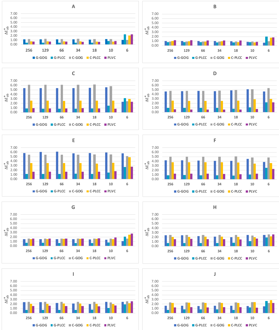
Fig. 7.3 The average \Delta E_{ab}^* for the Macbeth sample set for display A – J as a function of N (the number of linearisation samples).
