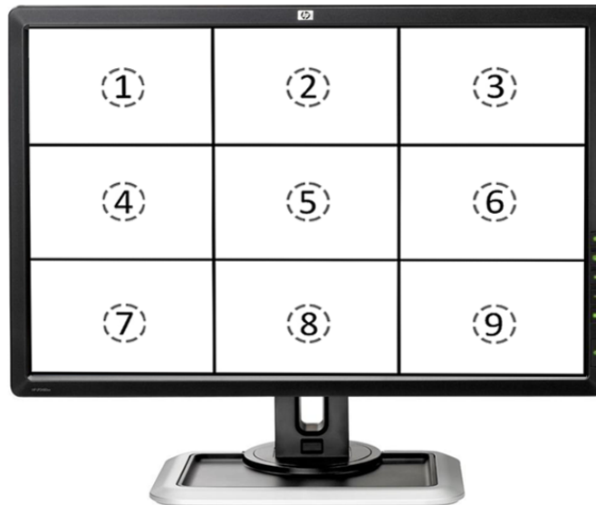
Fig. 5.5 Position of white measurements.
