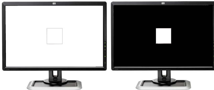
Fig. 6.2 Measuring the white over two different backgrounds to evaluate the Spatial Independence.
