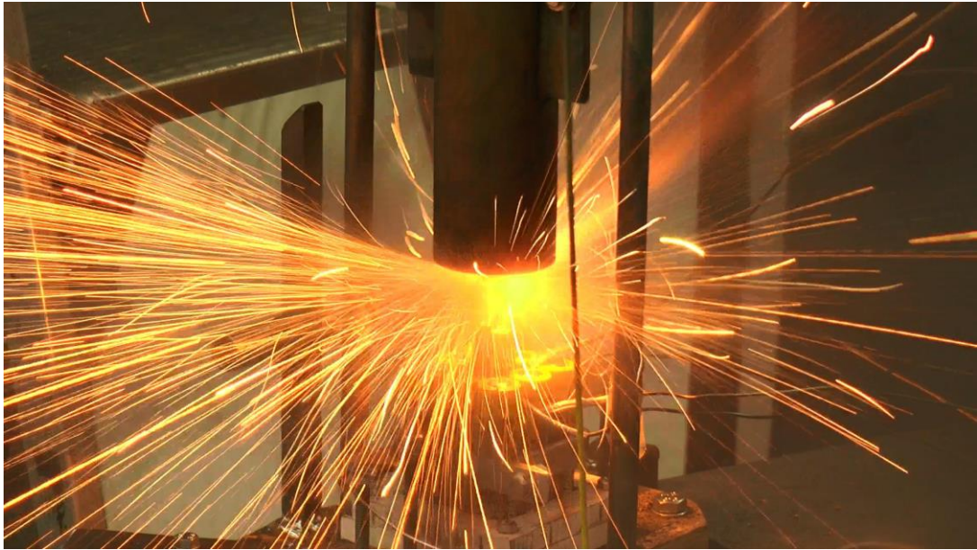
Figure 5.48: Fire sparks were produced after the impact.
