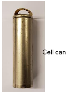
Figure 5.24: Remnant of the drained battery after the oven test.
