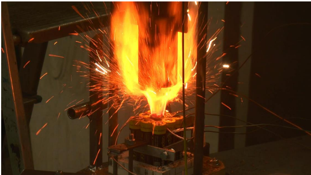
Figure 5.49: The cylinder was engulfed in fire.
