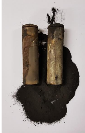
Figure 5.18: Aftermath of two-cell thermal runaway.
