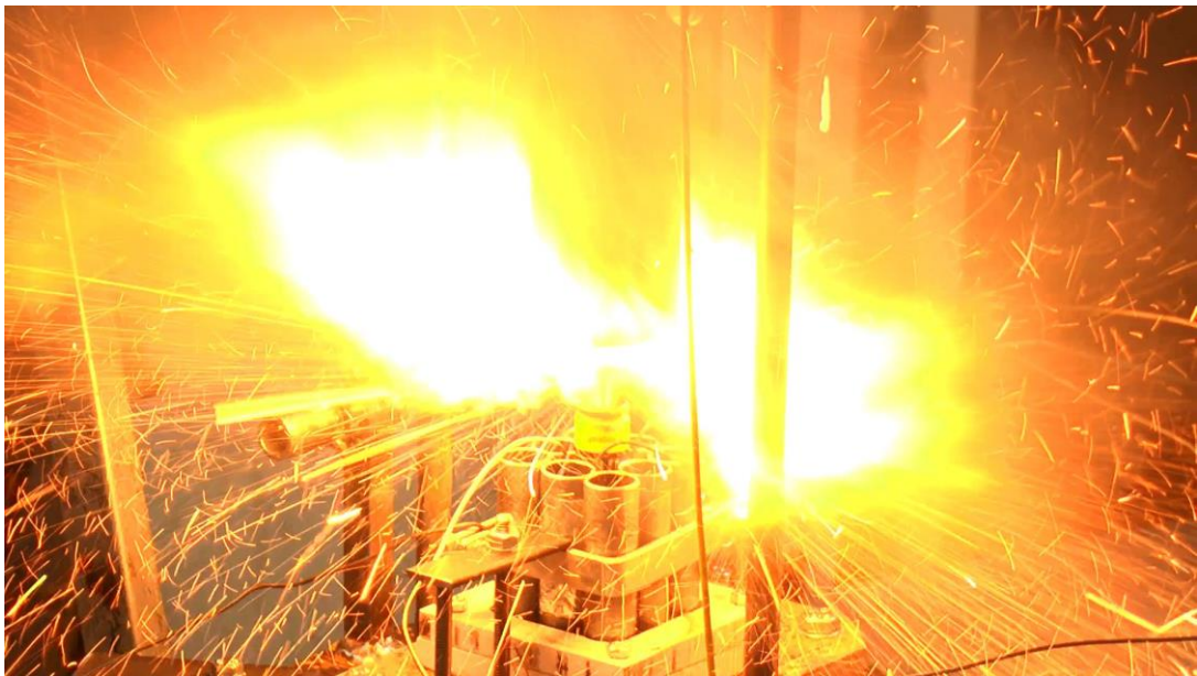
Figure 5.36: Fierce burning of the ejected gases.
