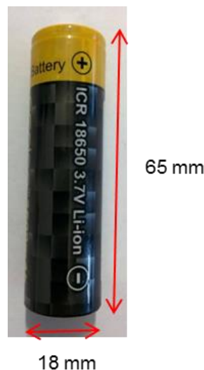
Figure 5.1: 18650 cylindrical lithium-ion cell used in the experimental work.
