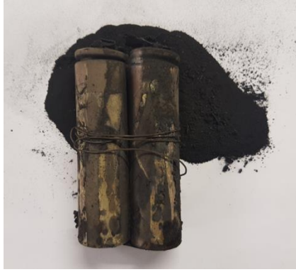
Figure 5.20: Aftermath of thermal runaway of two full-charged batteries connected in parallel.
