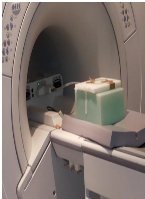
Fig. 5.31 The coil only measurement system demonstrated within a 1.5T MRI scanner
