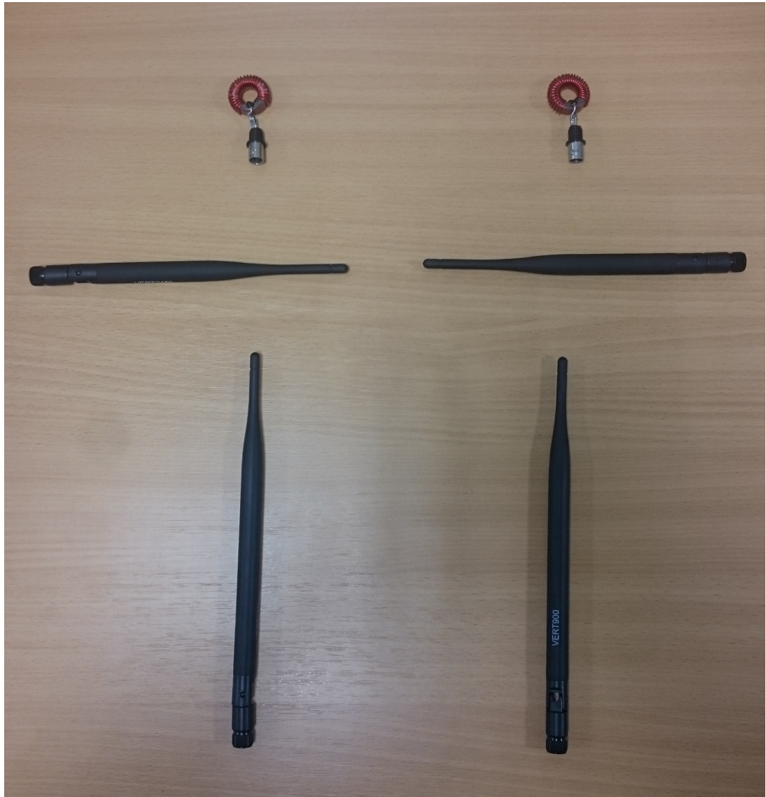
Figure 7.9: These are the three main antenna configurations used. From top to bottom: The toroidal choke coils; the whip antennas in ‘horizontal’ point-to-point transmission (longitudinal); the whip antennas in ‘vertical’ parallel transmission, this is optimal and is used for conventional signal transmission.
