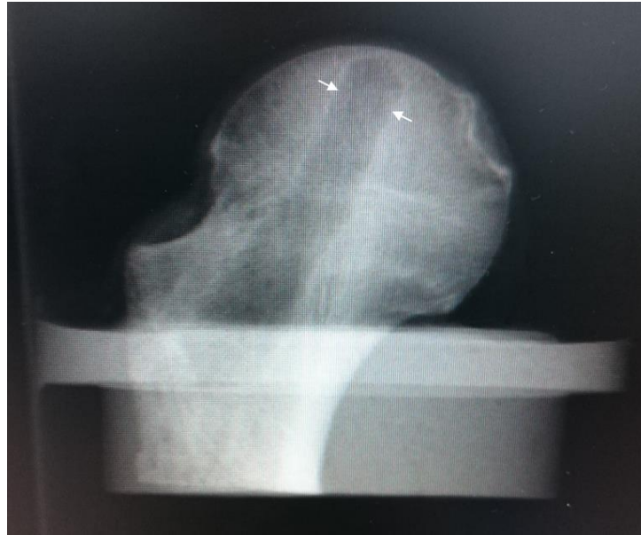
Figure 59 CT-scan of a potted sample with a simulated drilled lesion in the subchondral region of the femoral head (white arrows) administered through the femoral neck.
