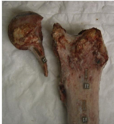
Figure 85 A typical picture of the neck fracture of a mechanically tested femur. Image from Tanck et al. (2009) reproduced with permission from Elsevier.
