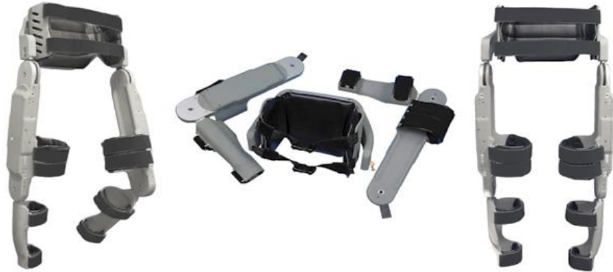
Figure 2.12 Vanderbilt Exoskeleton (Farris et al., 2012).
