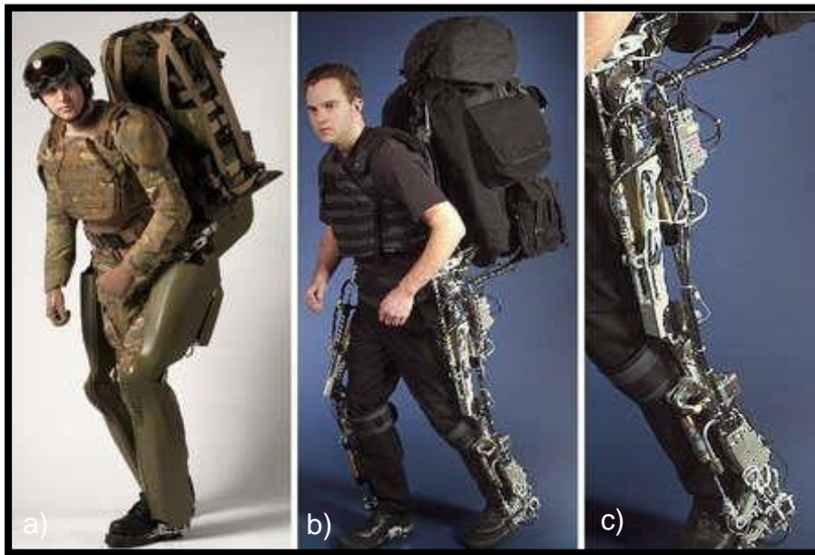
Figure 2.8 BLEEX Exoskeleton(Zoss et al., 2006) a)BLEEX close to finish product with cover, carrying backpack load b) BLEEX prototype mechanical design with engine and payload at the back c) BLEEX joint and hydraulic actuation system
