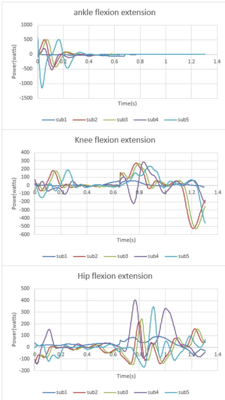
Figure 7.1 The power consumption simulated for the exoskeleton according to the subjects angular velocities at the sagittal plane joints of ankle, knee, and hip.
