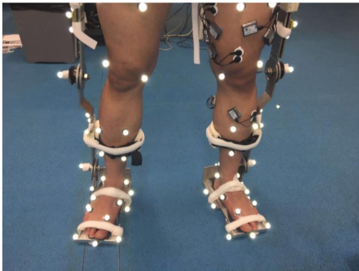
Figure 6.2 Exoskeleton shoe, ankle and knee motion capture experimental setup front view
