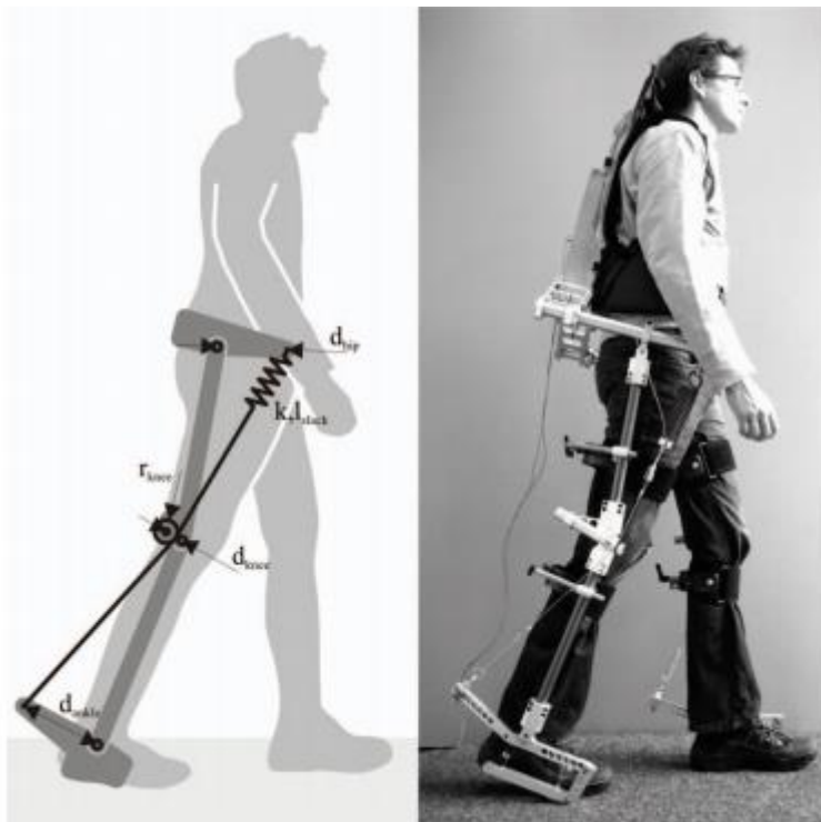
Figure 2.15 XPED2 artificial tendon exoskeleton design (Wang et al., 2011)
