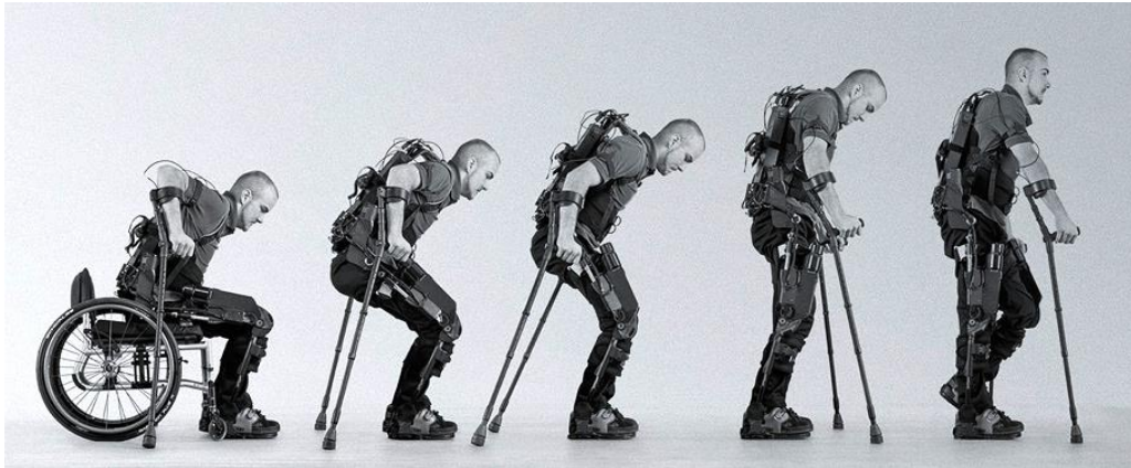
Figure 2.11 eLEGS Exoskeleton (bionics, 2017)
