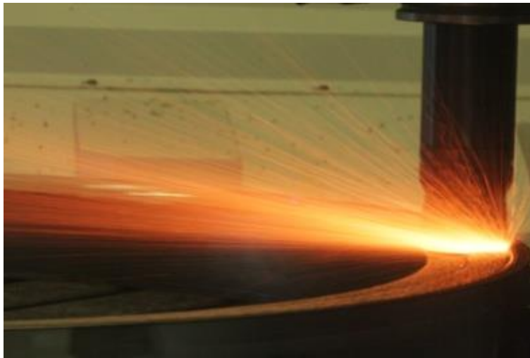
Figure 1.2: High-speed dry milling process of nickel-based super alloy using SiAlON cutting tools.
