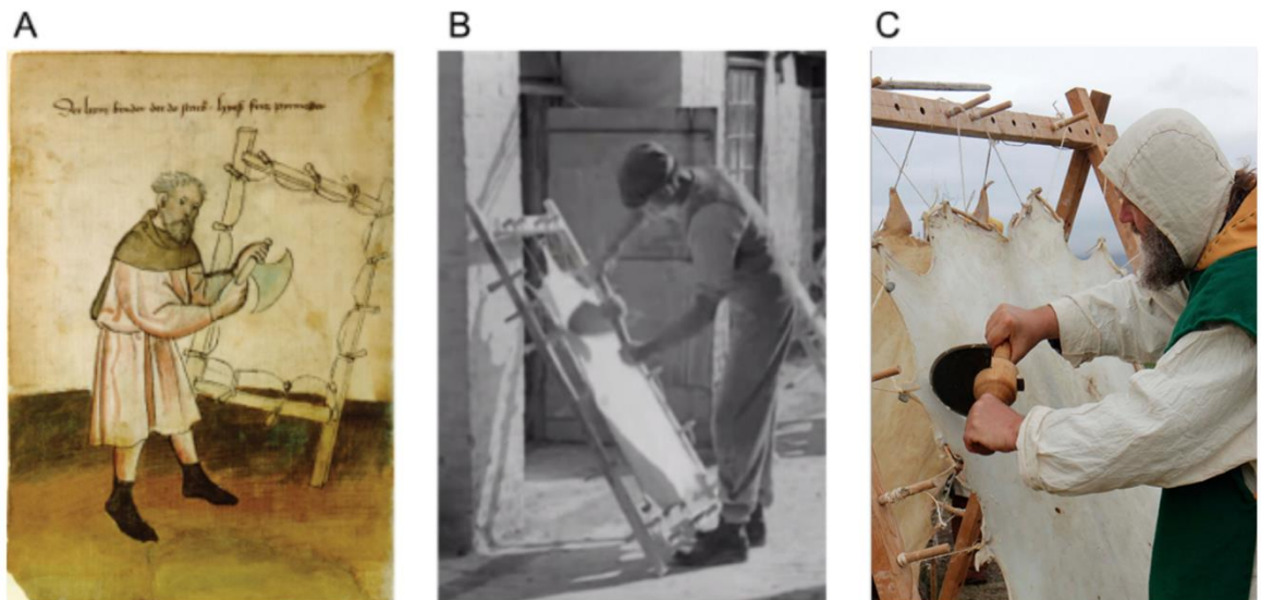
Figure 3.8: Shaving the parchment on the frame: A) Depiction of a parchment maker shaving the skin with a lunellum, Folio 34 Mendel Housebook c.1425, Amb. 317.2 ; B) Still from ‘The Very Idea’ , 1939 (British Pathé) from a parchment makers in Brentford, Middlesex; C) J. Vnouček embodying Mendel’s parchment maker nearly 600 years later (courtesy of J. Vnouček)
