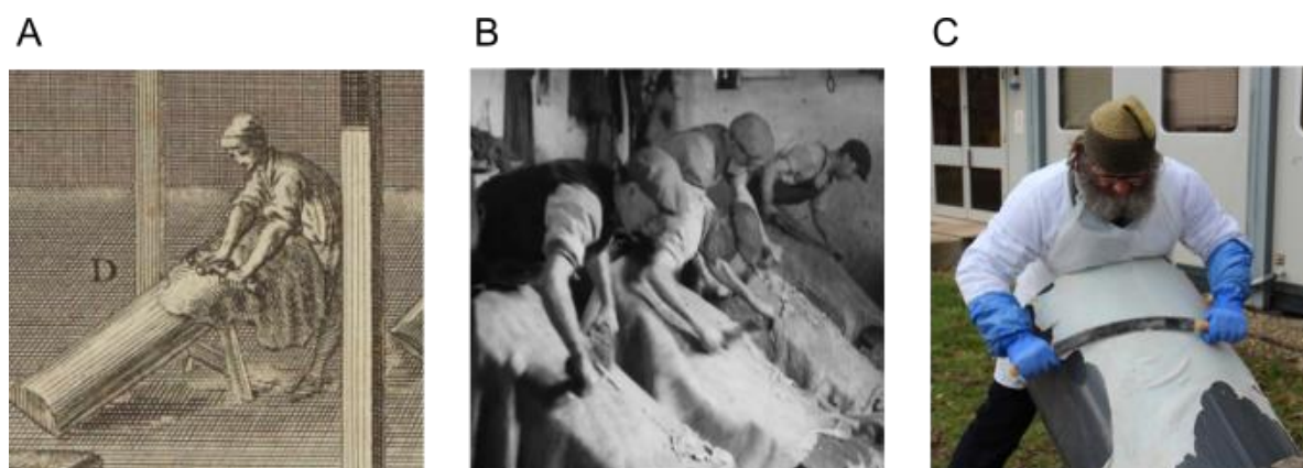
Figure 3.6: Unhairing and fleshing on the beam: A) Detail from Plate I, Lalande 1762, showing the unhairing of the skin; B) Still from ‘ The Romance of Leather ’, capturing workers from Richard Hodgson & Sons Tannery, Beverley, E. Yorkshire, fleshing skins on the beam; (Debenhams 1932) C) A skin from this study being unhairing and fleshing in the same manner using the traditional double-handed curved knife (by S. Doherty)
