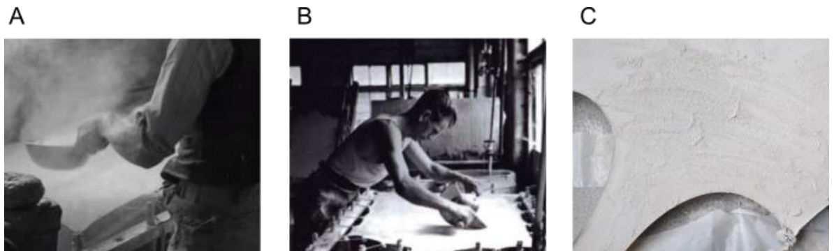
Figure 3.9: Degreasing: A) Still from 'The Very Idea', 1939 (British Pathé) showing boiling water being poured onto both the hair- and flesh-side of the parchment while still on the frame, followed by scraping; B) Photo of degreasing and scraping with the aid of boiling water at Messrs. Russell Leather & Parchment Works, Hitchin, Hertfordshire, c. 1930s (Hampshire County Council 2008); C) In this study, chalk was also applied to the flesh-side to help draw out the grease and improve the whiteness of the finished parchment (by S. Doherty)
