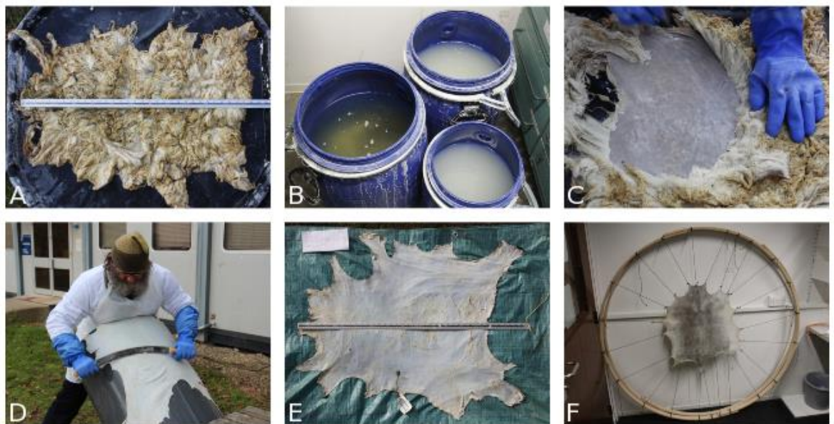
Figure 5.1: Method 1: A) salted skins are rehydrated and washed; B) skins are submerged in a lime solution; C) unhaired; D) fleshed on the beam; E) delimed in water; F) and dried under tension (by S. Doherty)
