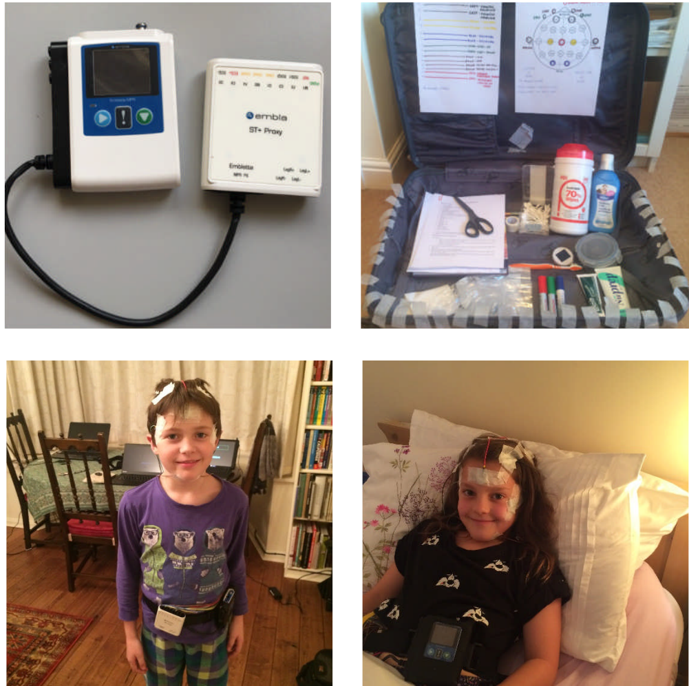
Figure 4.5 The Embla® Systems Embletta MPR + ST Proxy polysomnography equipment set up on two children and the consumables needed to apply the equipment.
