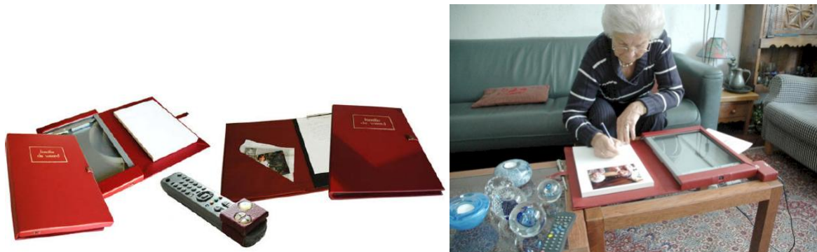
Figure 3.3 The working prototype consisting of a notebook with a scanner in its cover, and a small extension to the television's remote control.
