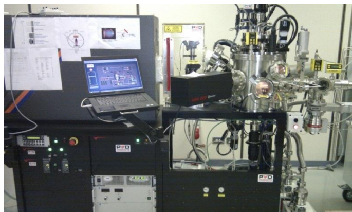
Figure 3.7: Picture of the PLD system used to prepare some of the thin films discussed in this thesis.
