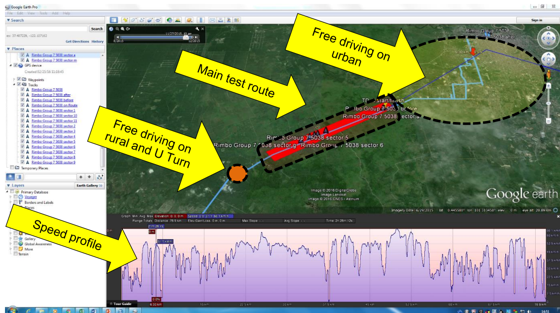
Figure 52: Visualization of GPS track and speed profile using GEP application
