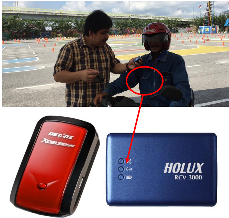
Figure 30: BT-Q1000eX and Holux RCV-3000 are a GPS receiver and data logger with 1Hz log rate
