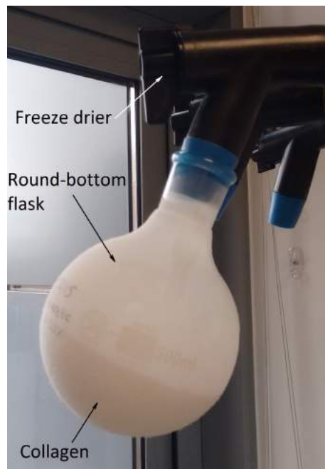
Figure 15: The collagen-acetic acid mixture was sublimated in the freeze drier to remove the acetic acid.
