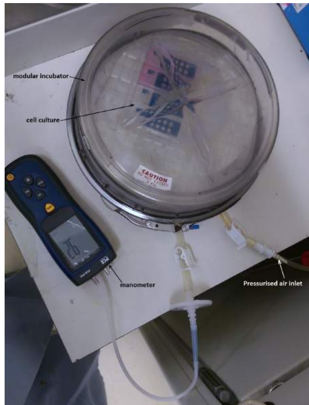
Figure 76: In the pressure model, a modular incubator is pressurised, using a manometer to monitor the pressure increase.
