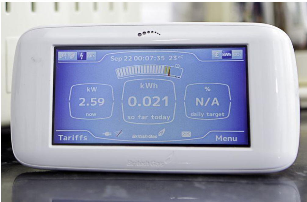
Figure 1-7: A typical domestic smart meter customer interface (Ivy Link 2015)
