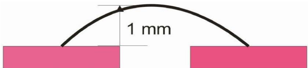
Figure 6.3 Orientation of the wire over the hole made in the appliance
