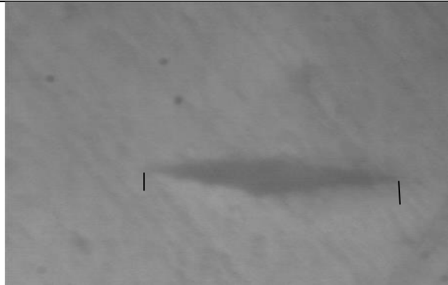
Figure 3.7 The indentation length in the enamel slab ( \mu\text{m} )
