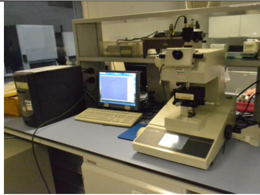
Figure 3.6 Microhardness computer-aided Duramin indenter machine (Struers A/D, DK 26-19, Denmark)
