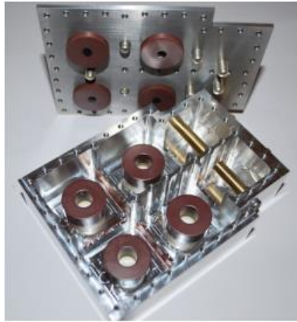
Figure 2-21: Prototype manufactured dielectric resonators, combline resonators and hybrid model [43]
