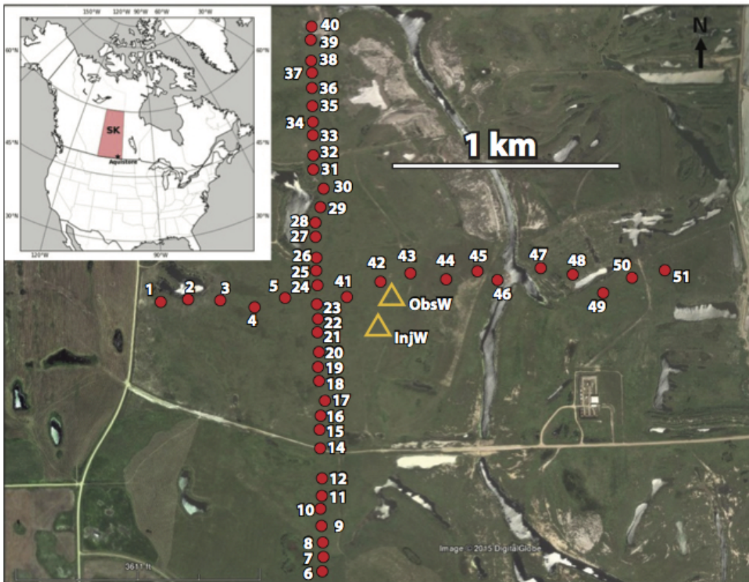
Figure 3.1: Permanent seismic array survey geometry at Aquistore \text{CO}_2 storage site in Saskatchewan, Canada. Geophones are denoted by red dots alongside the station number, while the observation and injection wells are illustrated by yellow triangles. (Appeared as figure 2 in (Birnie et al., 2016).)
