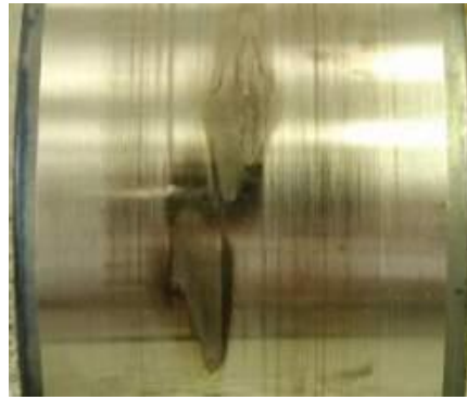
Figure 2-3. Adhesive wear occurred on the inner ring of a bearing (24)
