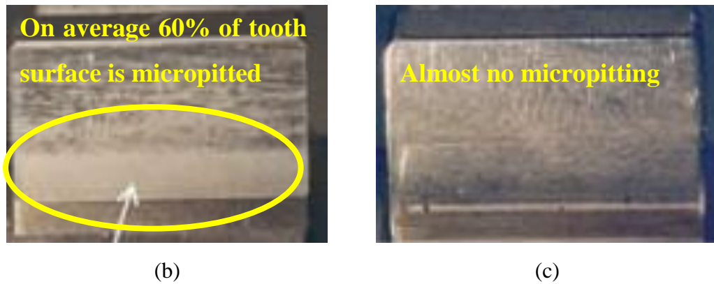
Figure 3-36. The effect of surface roughness treatment (superfinishing) on micropitting examined using a FZG gear tester based on test procedure described in "Test Procedure for the Investigation of Micropitting Capacity of Gear Lubricants," FVA Information Sheet 54/I-IV. a) Shows the micropitted area as a function of load stage and b and c) present the images from the baseline and superfinished gear teeth respectively (104)
