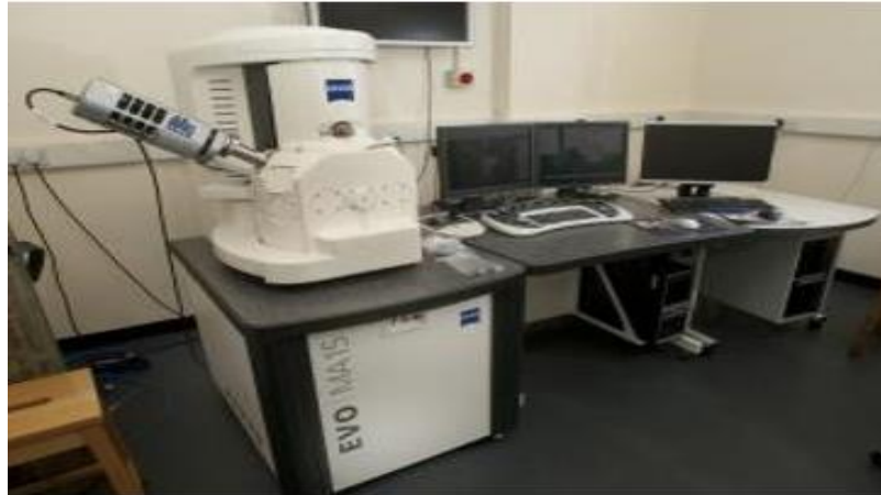
Figure 4-6. Carl Zeiss EVO MA15 Scanning electron microscopy and energy dispersive X-ray analysis setup
