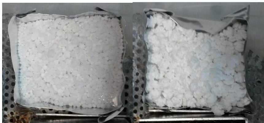
Figure 157. Anhydrous calcium chloride as desiccant, with the fresh powder shown on the left, and the expanded exhausted powder shown on the right
