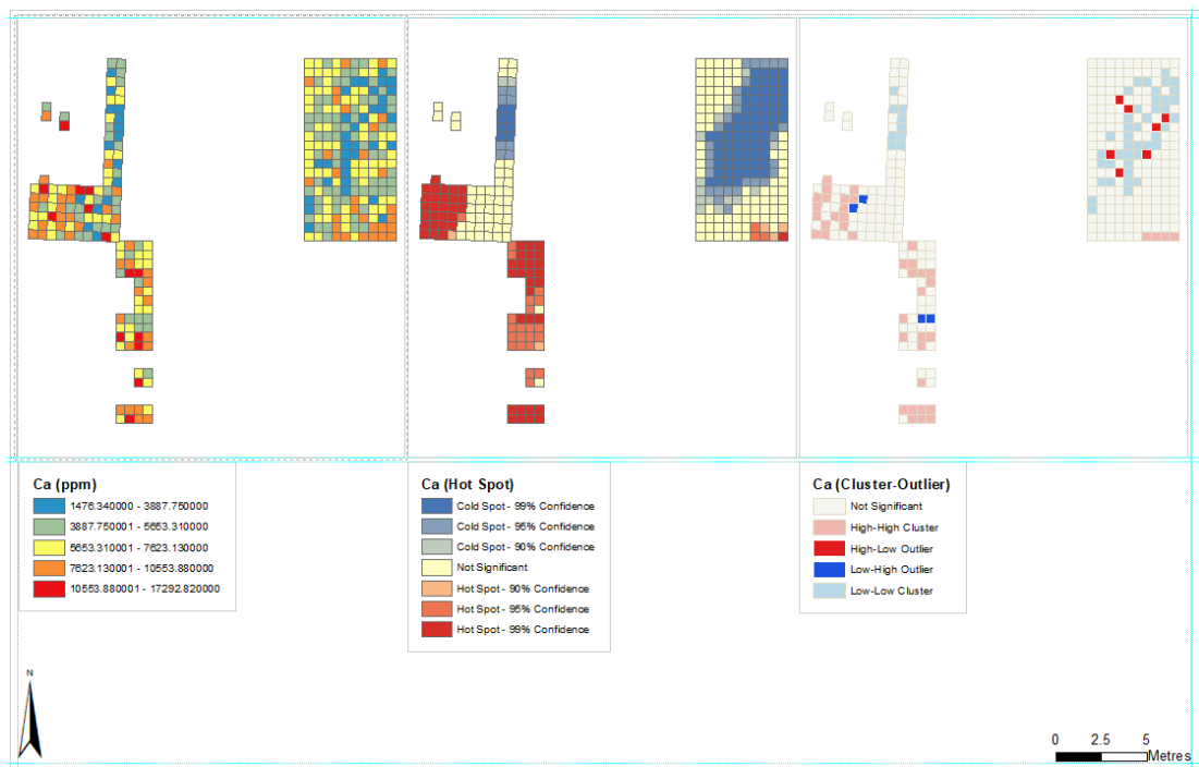
Figure 103. Simple, HSA and C-OA plots of readings from FpXRF for calcium
