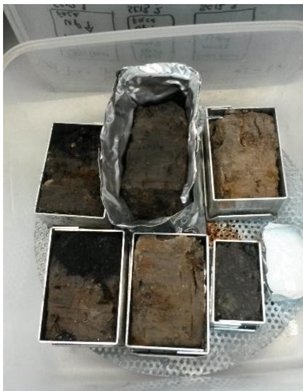
Figure 156. Acetone vapour exchange setup for drying micromorphology tins from Flixton Island 2 and Star Carr, with a pot of anhydrous calcium chloride as desiccant on right end of the bottom row in the photograph.
