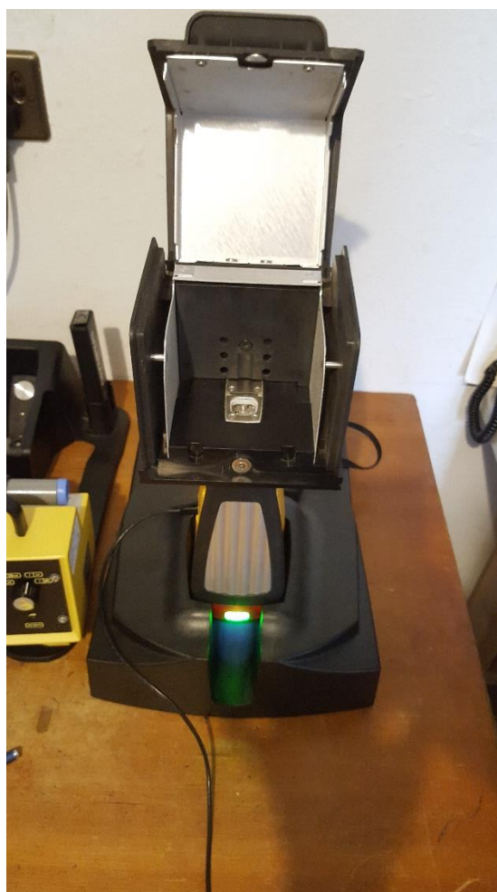
Figure 83. Vertical setup for the Olympus Flex Stand, looking down on the stand, with the lid of the chamber lifted to show inside the chamber and the analysis window.
