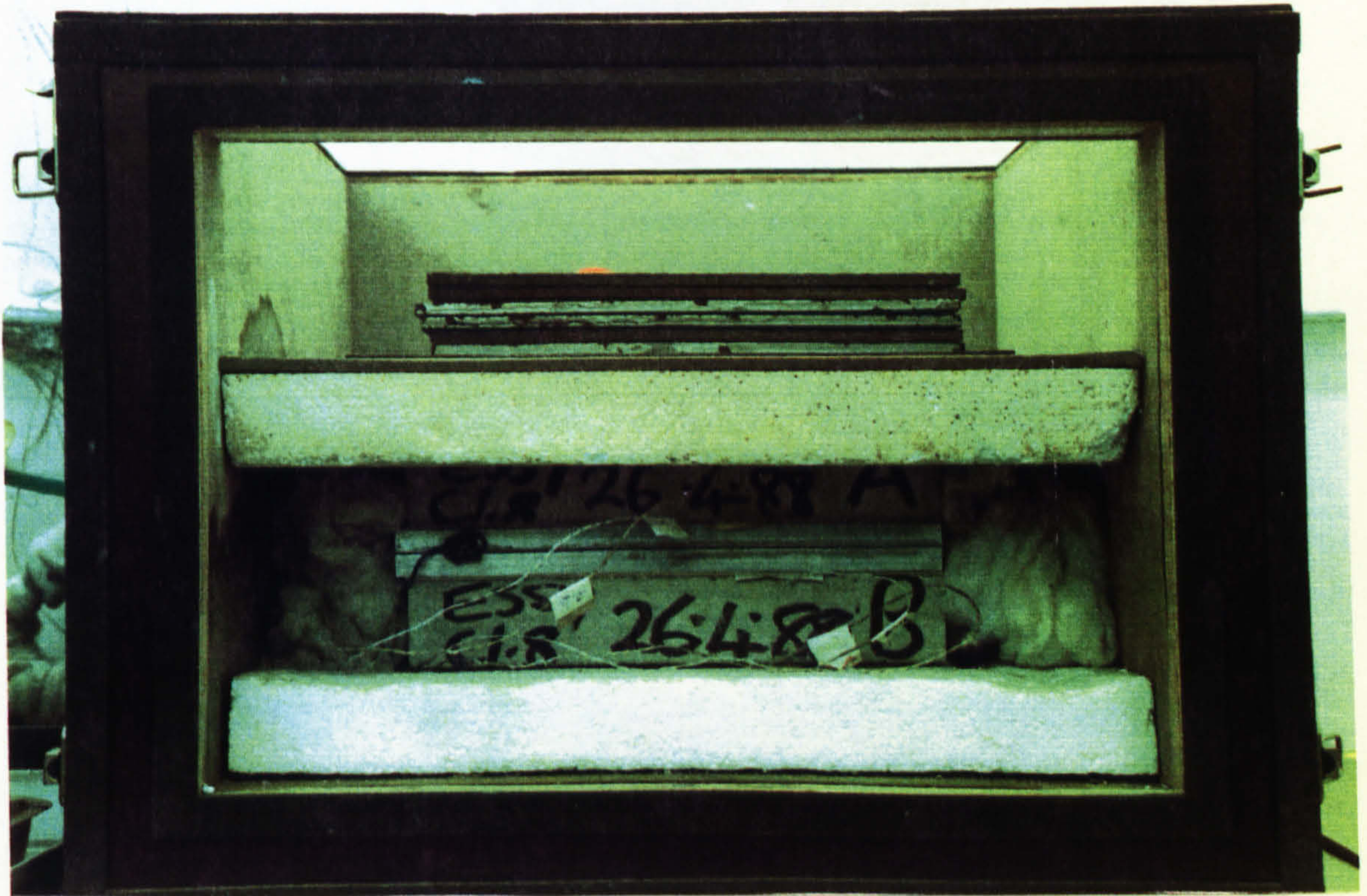
Fig.(5.4) Photograph of opened insulating cabinet.
