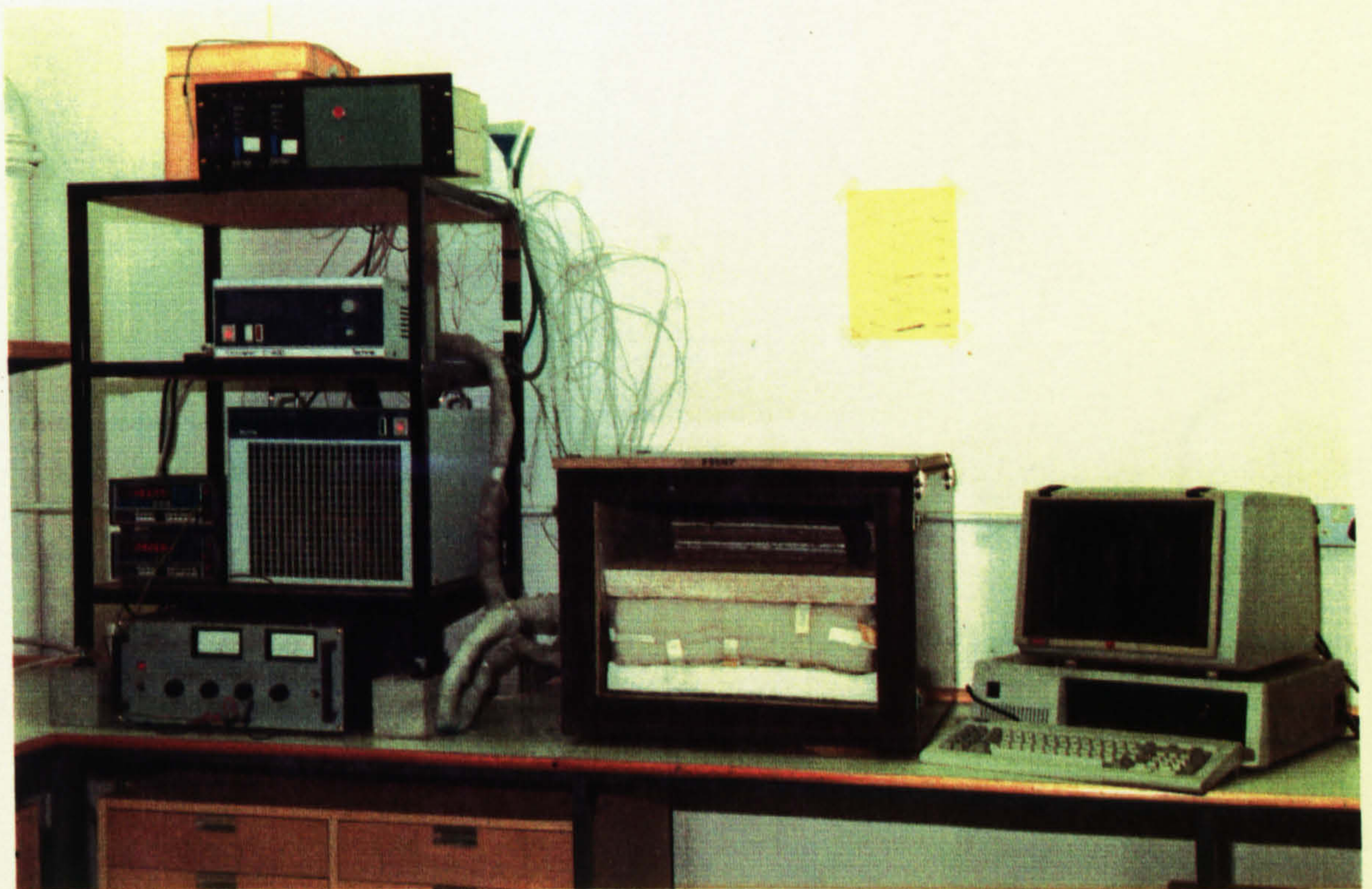
Fig (5.5) Photograph of the Hot-plate Apparatus and Insulating Cabinet with controlling equipment and the micro-computer.
