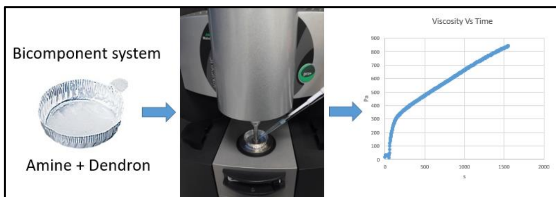
Figure 2-17 General scheme of the process of collecting a progression of viscosity from solution state of components to the sol-gel transition triggered by the addition of the second component.
