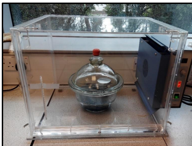
Figure 3-16 The diffusion chamber (desiccator) inside an incubator to maintain a stable temperature. Notice that the closed system (chamber) maintains rich the vapour pressure of toluene so gels don't dry out.
