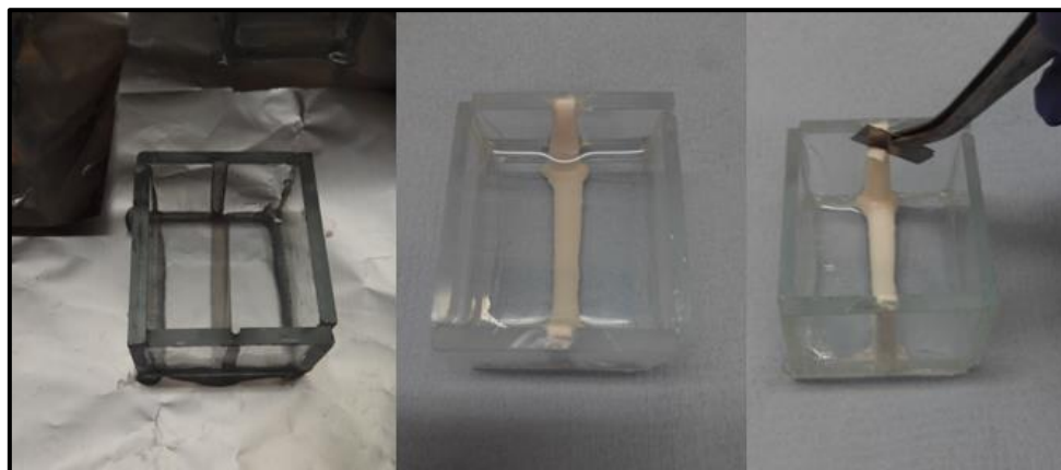
Figure 3-18 The process of filling the central hole with white silicone in order to seal one side from the other with an aluminium barrier. Once silicone is in contact with toluene it swells and there was therefore a need to removing the excess of swollen white silicone with a very sharp blade to obtain a completely flat surface in the diffusion cell.
