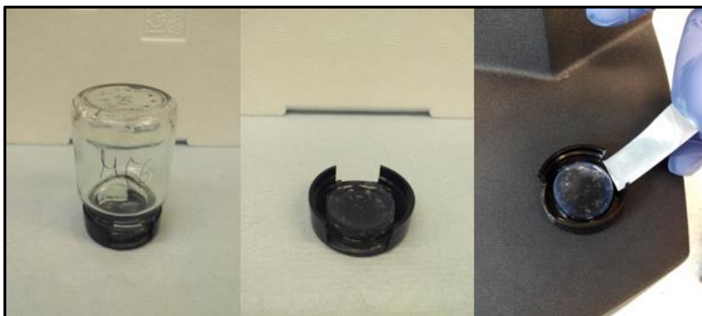
Figure 4-15: Procedure of preparations of disc of gels. The obtained disk can be handled in one piece until it is placed in the rheometer for testing.
