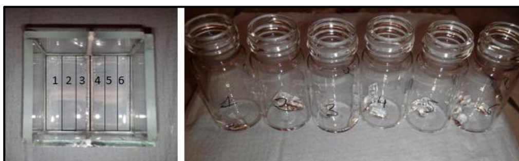
Figure 6-18 Diffusion cell divided in each region (left) and the collection of the material corresponding to those regions in 8 mL vials.
