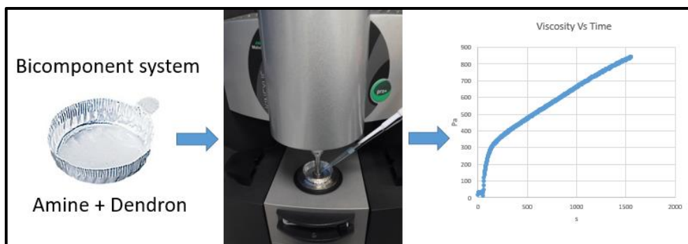
Figure 6-15 example of the set up where gels are introduced in liquid state and there is a transition to gel produce either the addition of a second component or the lowering of the temperature.
