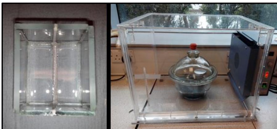
Figure 6-17 Diffusion Cell (left) with the two sides easily observed and an incubator with the diffusion chamber filled with several diffusion cells performing the experiment at controlled temperature.
