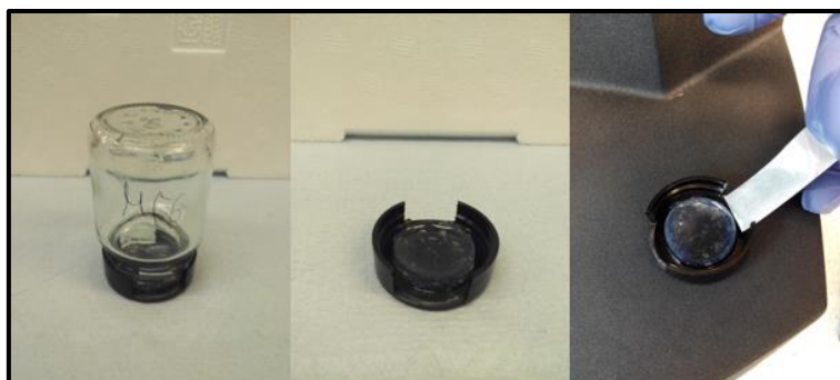
Figure 6-14 Process of placing a formed gel inside a Jar and the careful extraction of it to the rheometer testing platform.
