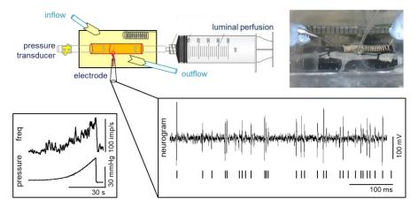
Figure 2: Schematic and photograph of the experimental setup. For description refer to the text.
