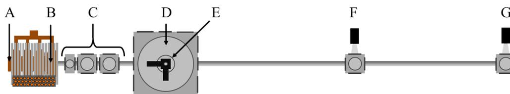
**Figure 3.28:** Schematic illustration of the UED apparatus at SLAC showing the RF electron gun (A), the main solenoid (B), the beam diagnostic module (C), the diffraction chamber (D), the sample delivery system (E), the near detector (F), and the EMCCD far detector (G).
