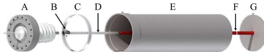
**Figure 3.27:** CAD drawing of the enclosure surrounding the high-voltage feedthrough in the TRED apparatus electron gun, showing the HV feedthrough (A), HV connector (B), the PTFE flange fitting (C), the HV cable (D), the steel cylinder enclosure (E), the PTFE cable fitting (F), and end plate (G).
