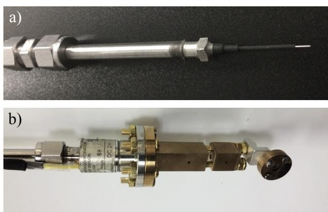
**Figure 3.25:** Photograph of the TRED apparatus a) effusive and b) pulsed nozzle.
