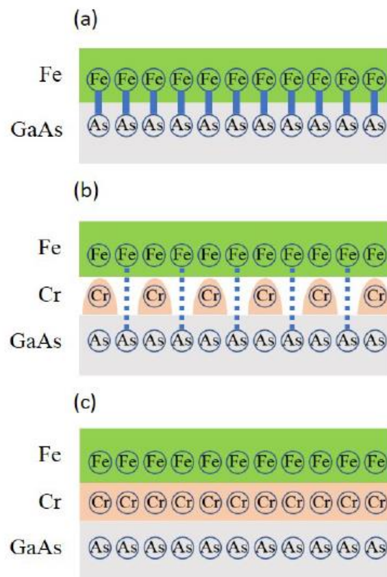
Figure 5.10 indicates the influence of the Cr interlayer between the Fe-As bonding.
