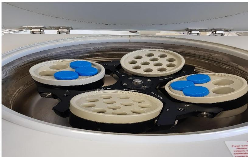
*Figure 2.6: Bench Centrifuge (temperature controlled).*
