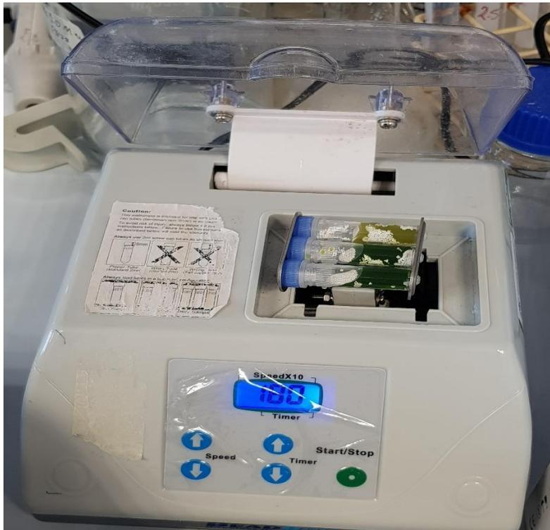
*Figure 2.2: Beadbug Microtube homogenizer for disruption of algal cells.*
